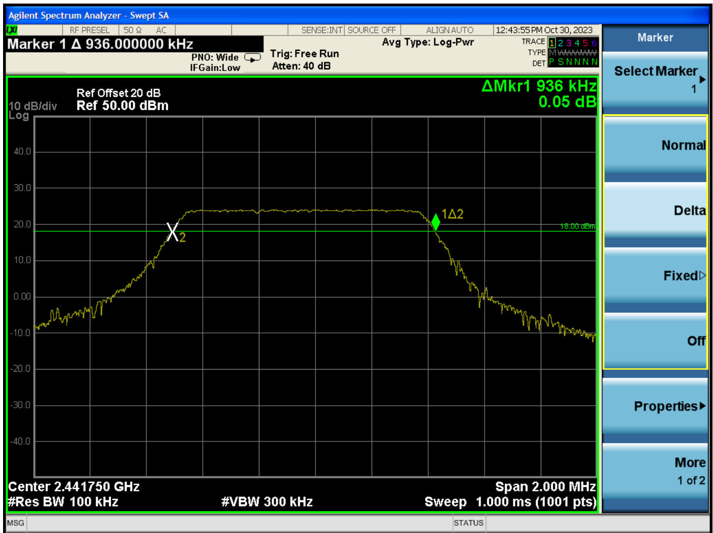
DTS Bandwidth – Middle Channel
