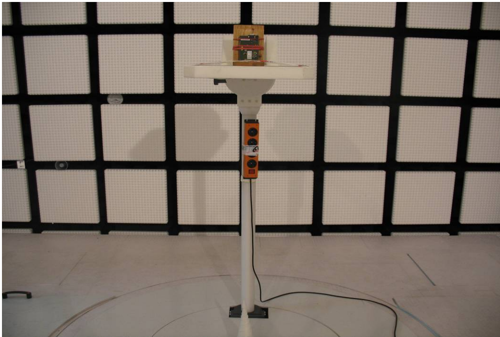
Photo 3: Pre-scan position for spurious radiated measurements >1GHz
