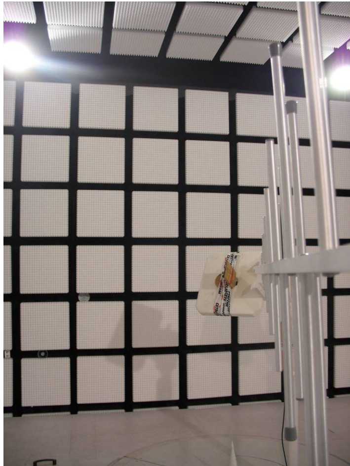
Photo 7: Position for max. E.I.R.P. (GFSK) DUT 55° / Azimuth 130°
