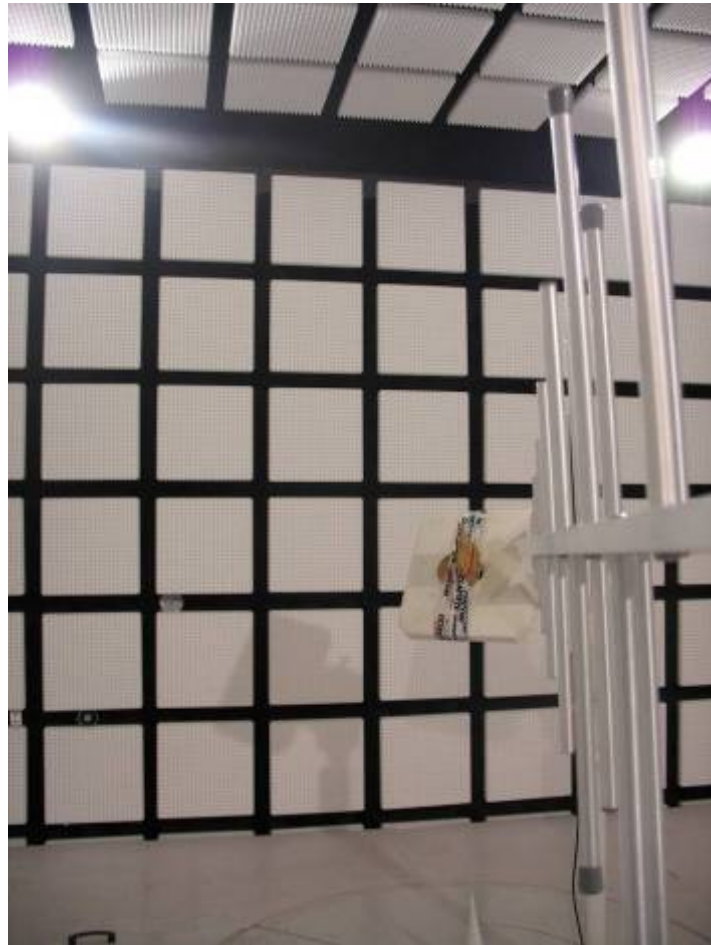
Photo 7: Position for max. E.I.R.P. (GFSK) DUT 55° / Azimuth 130°
