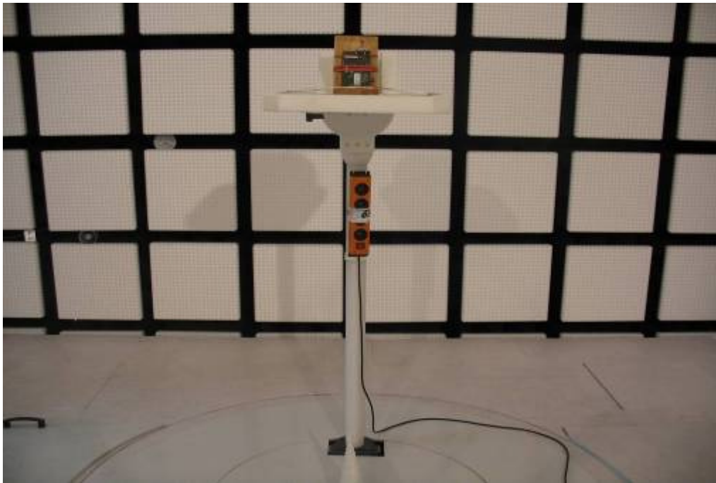
Photo 3: Pre-scan position for spurious radiated measurements >1GHz
