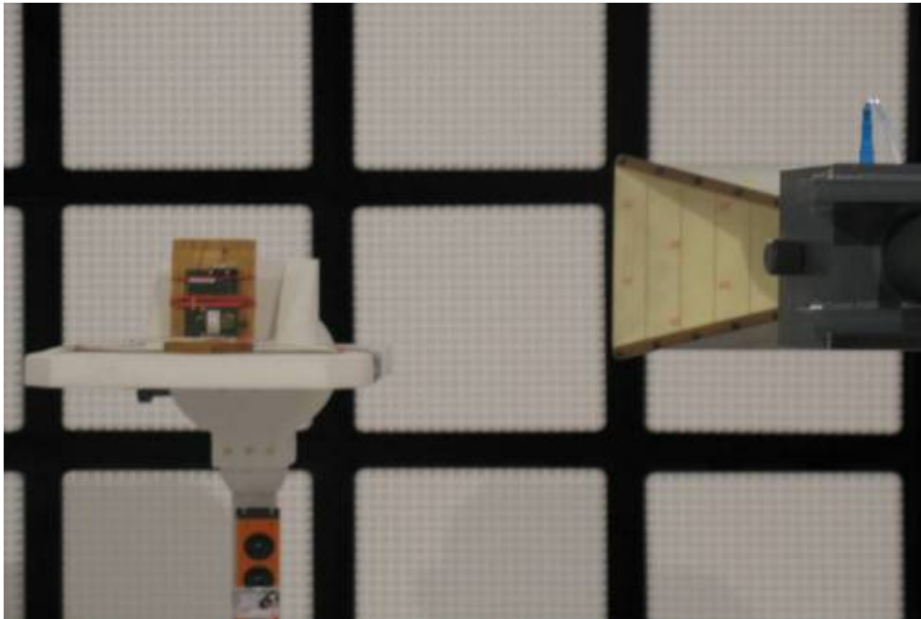
Photo 5: Pre-scan position for spurious radiated measurements >1GHz
