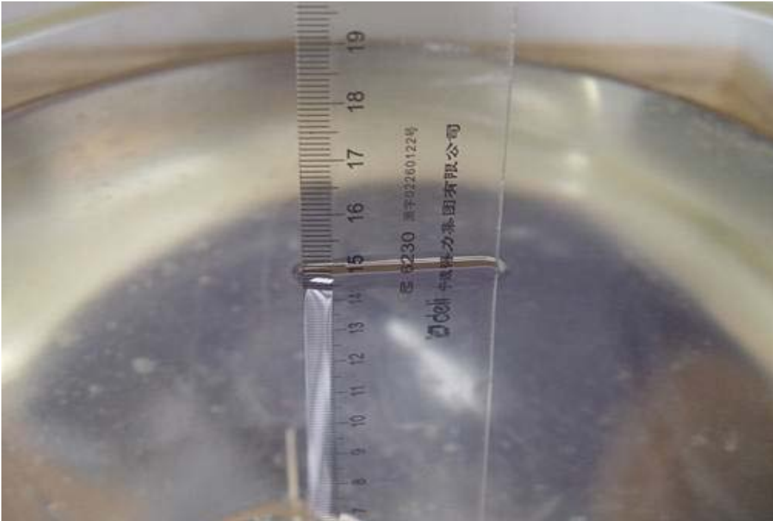
Photo of Liquid Height for Head SAR
