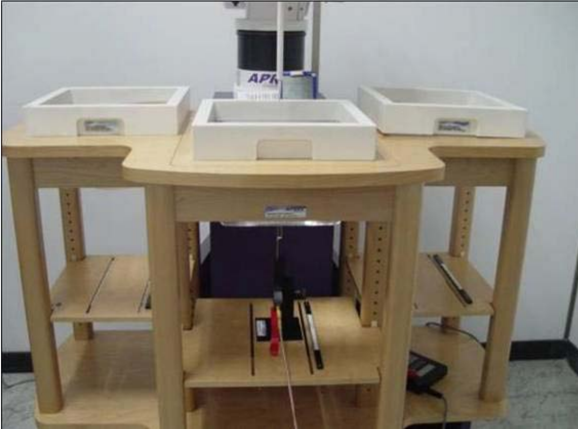
Photo of Liquid Height for Head SAR
