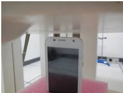
Body position Top with gap 10mm
