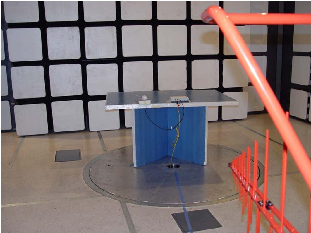
Radiated Emissions <1 GHz (dc Powered)
