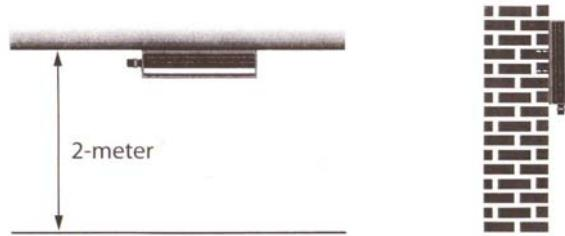
Place indoor antenna at least 2 meter distance from ground enable to get better service range; The location should be placed in the center of the building floor to be serviced by the unit.
