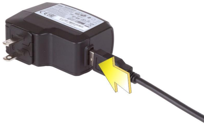
Figure 3-3: Connecting the MODAT-550A to the Power Adapter
