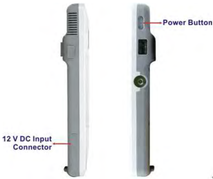
Figure 3-22: Power-up the System
