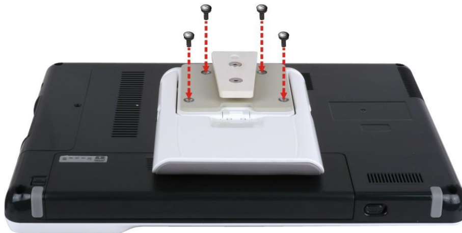
Figure 3-4: Installing the Mounting Bracket
