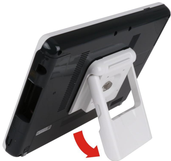
Figure 3-6: Adjusting the Tablet Stand
