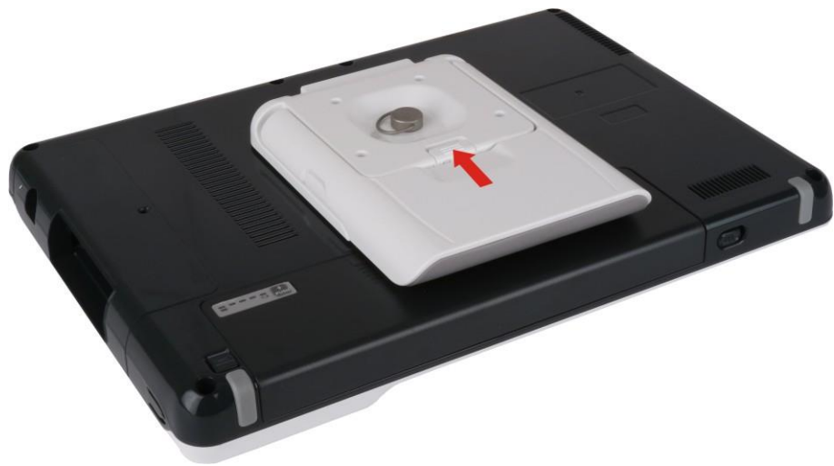
Figure 3-5: Releasing the Tablet Stand
