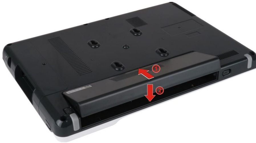
Figure 3-2: Battery Pack Installation
