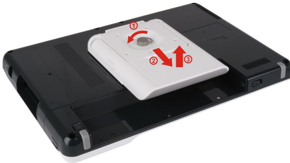
Figure 3-1: Removing the Tablet Stand Kit
