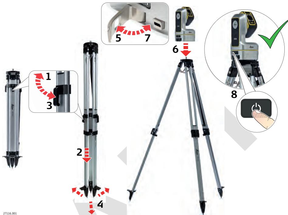
1. Open the latch from the tripod legs.
