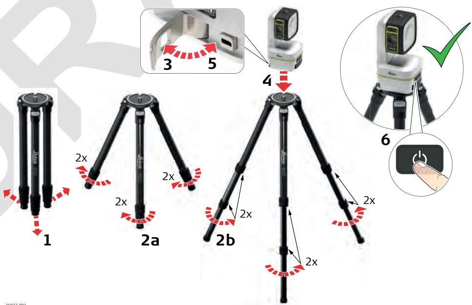
1. Unfold the legs of the tripod.
