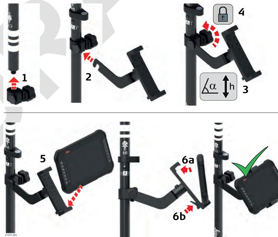
1. Insert the pole into the clamp hole.
