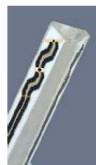
Figure 3.3 Probe Thick-Film Technique
