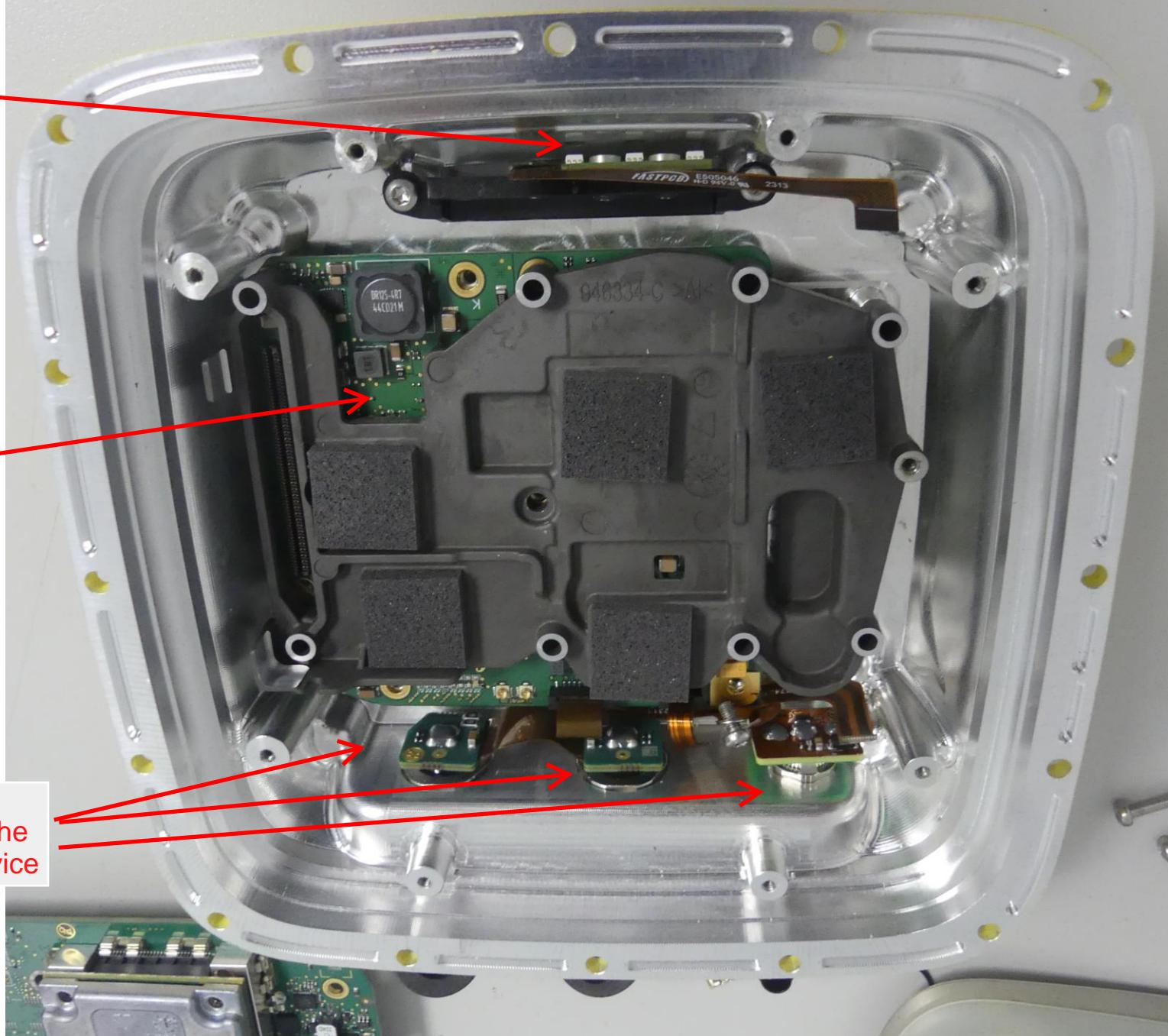
PCB of the connectors at the back of the device
