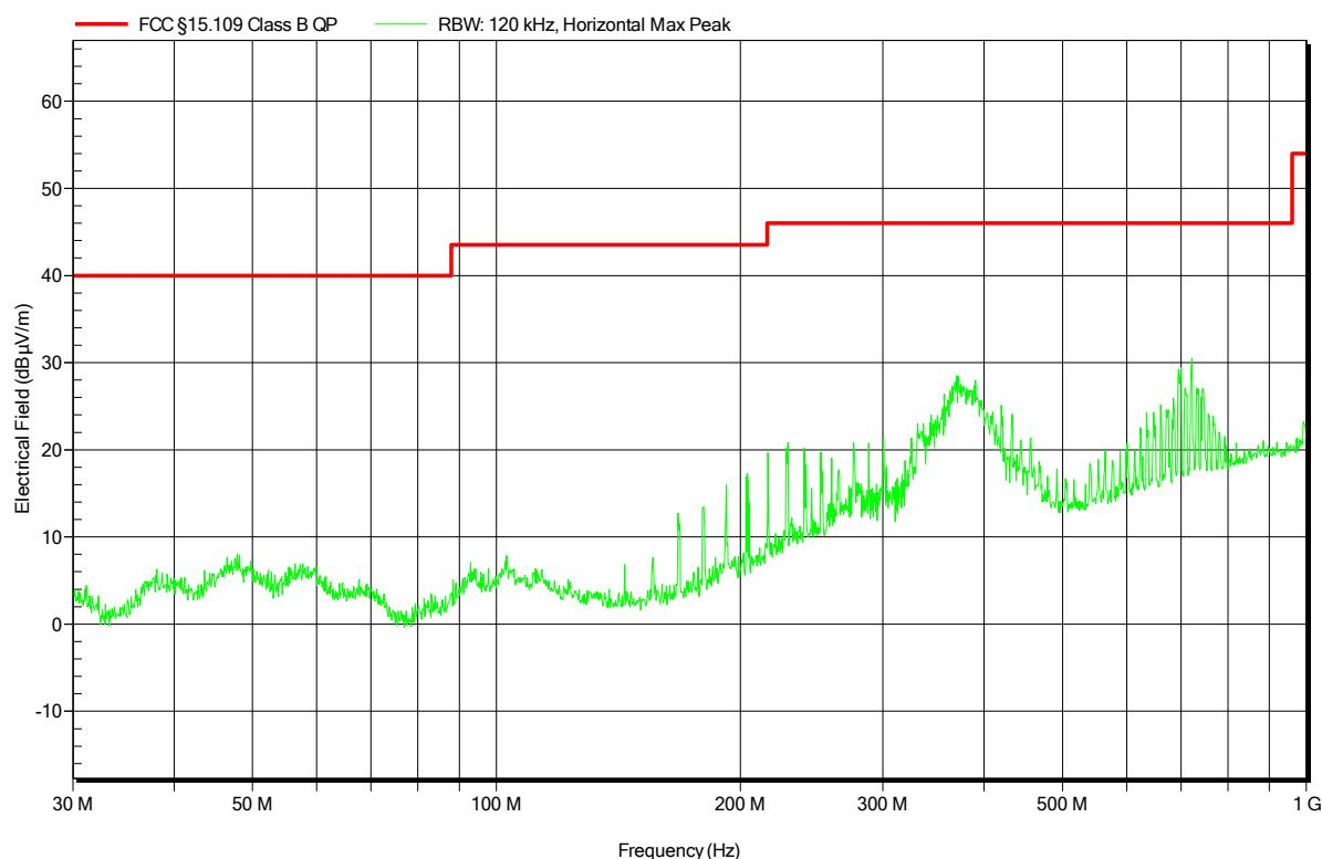
**Spurious emissions under normal conditions according to FCC 47 CFR 15.107 / ICES-003**
