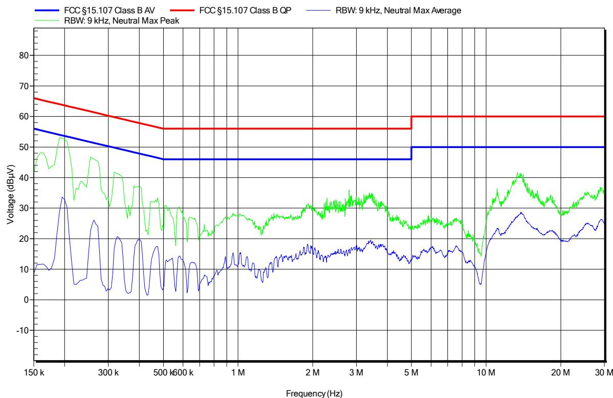
**EMI voltage test in the ac-mains according to FCC 47 CFR 15.107 / ICES-003**
