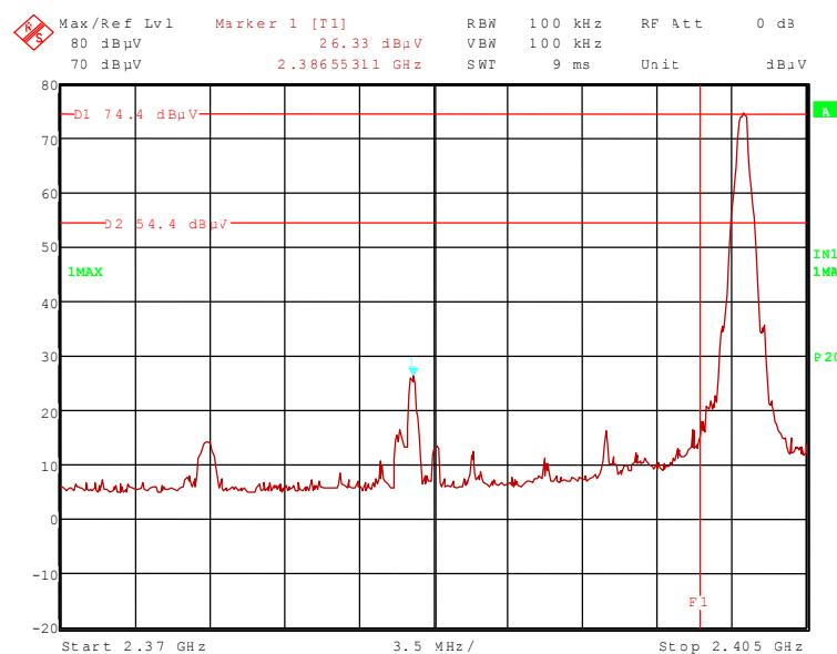
111592\_16.wmf: Radiated band-edge compliance, lower band edge, hopping on (operation mode 4):
