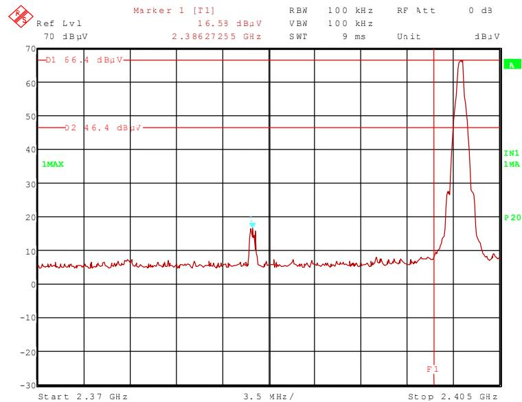
111592\_4.wmf: Radiated band-edge compliance, lower band edge, hopping on (operation mode 4):
