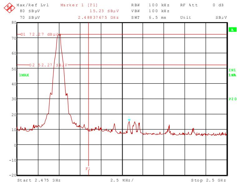
111592\_109.wmf: Radiated band-edge compliance, upper band edge, hopping on (operation mode 4):
