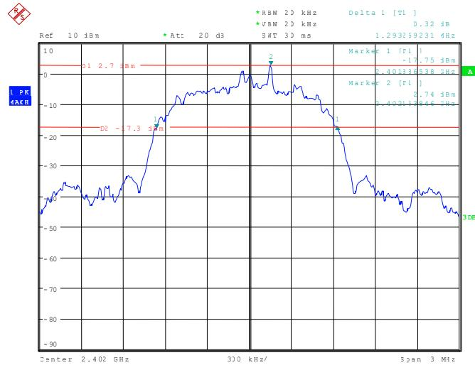
111592\_224.wmf: 20 dB bandwidth at the middle of the assigned frequency band:
