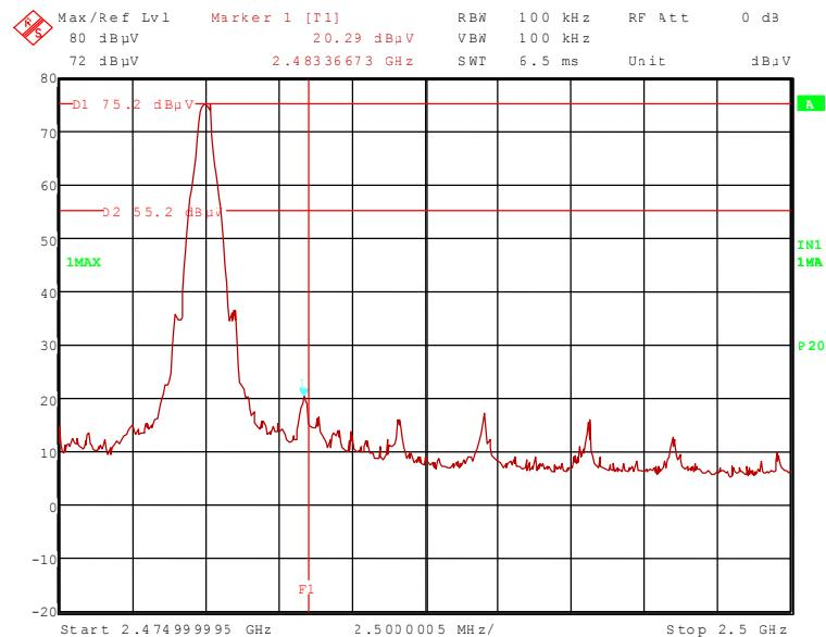
111592\_17.wmf: Radiated band-edge compliance, upper band edge, hopping on (operation mode 4):
