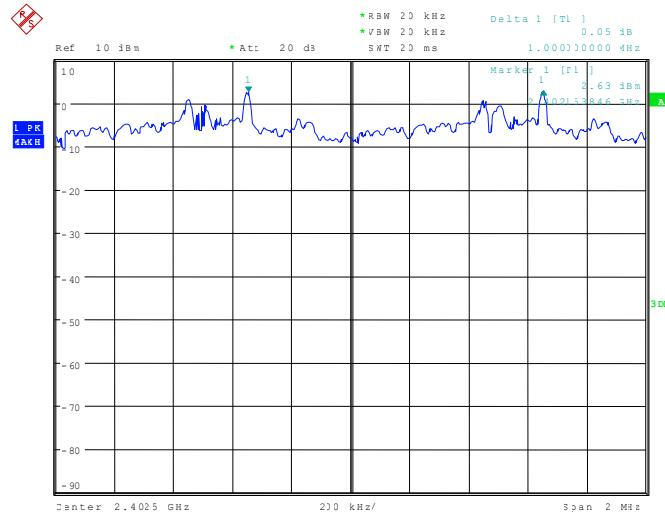
111592\_230.wmf: Channel separation at the middle of the assigned frequency band:
