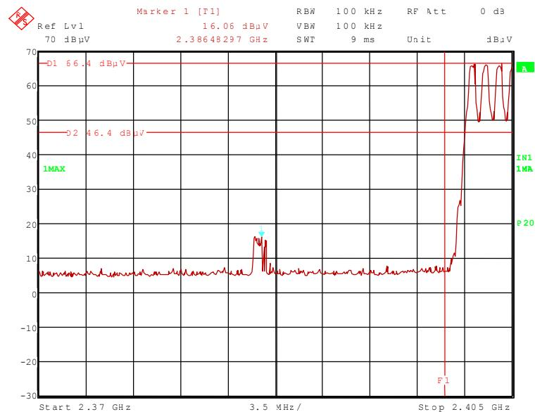
111592\_6.wmf: Radiated band-edge compliance, upper band edge, hopping off (operation mode 3):
