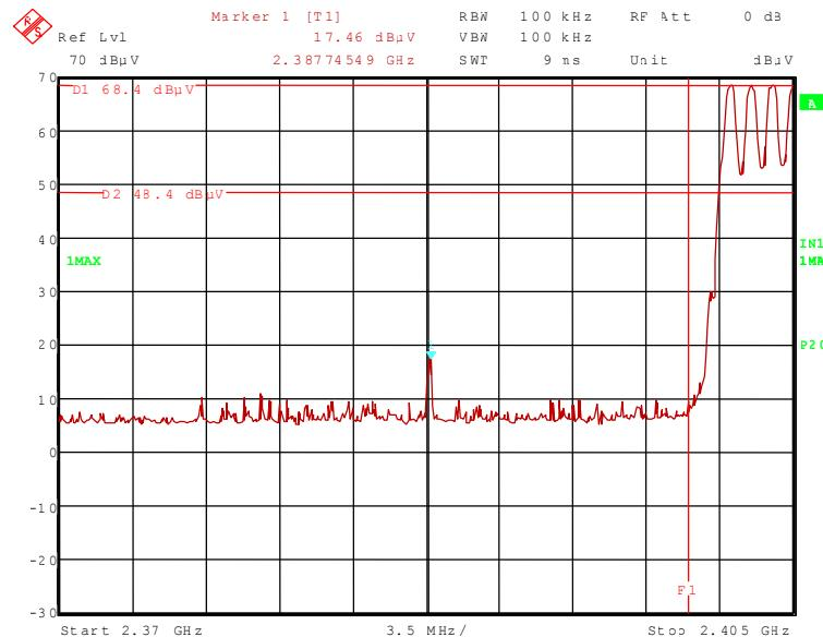
111592\_108.wmf: Radiated band-edge compliance, upper band edge, hopping off (operation mode 3):
