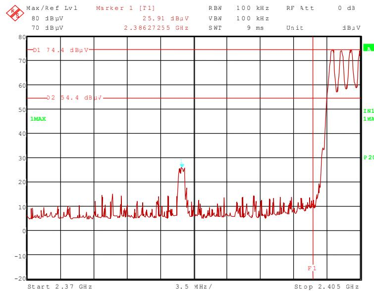
111592\_12.wmf: Radiated band-edge compliance, upper band edge, hopping off (operation mode 3):
