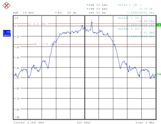
111592\_225.wmf: 20 dB bandwidth at the upper end of the assigned frequency band:
