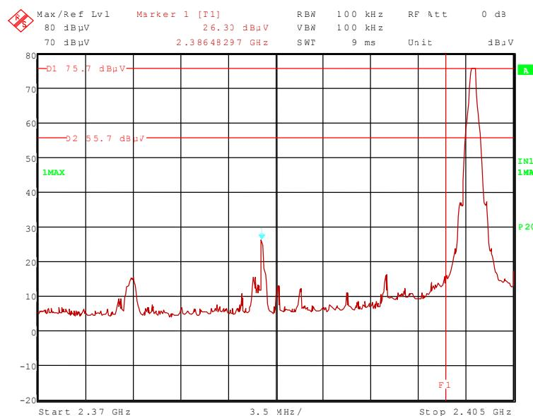
111592\_29.wmf: Radiated band-edge compliance, lower band edge, hopping on (operation mode 4):
