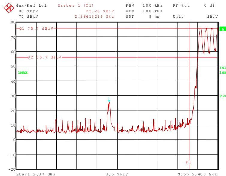
111592\_25.wmf: Radiated band-edge compliance, upper band edge, hopping off (operation mode 3):
