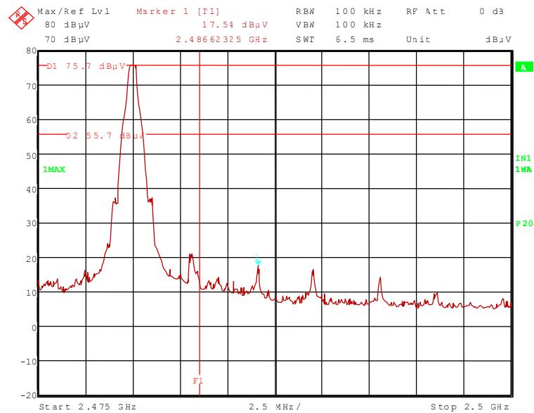
111592\_30.wmf: Radiated band-edge compliance, upper band edge, hopping on (operation mode 4):
