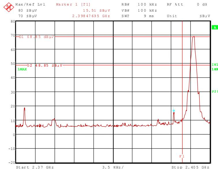
111592\_110.wmf: Radiated band-edge compliance, lower band edge, hopping on (operation mode 4):
