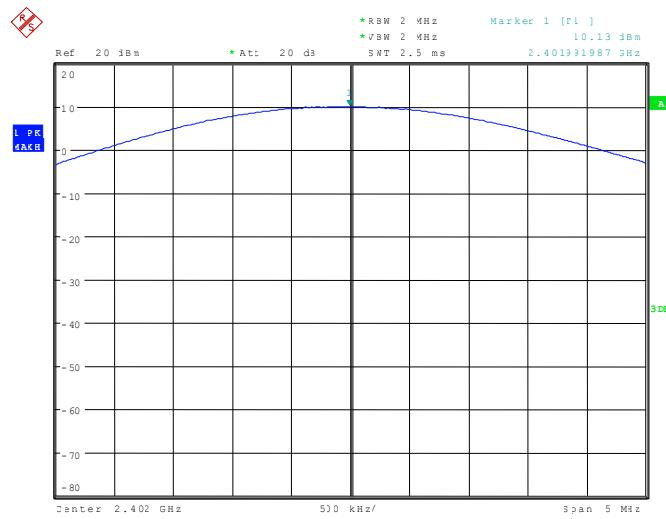
111592\_242.wmf: Maximum peak output power at the middle of the assigned frequency band (operation mode 2):
