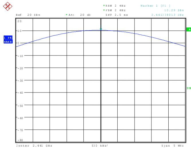
111592\_243.wmf: Maximum peak output power at the upper end of the assigned frequency band (operation mode 3):
