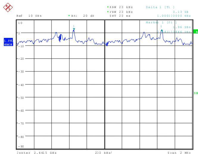
111592\_231.wmf: Channel separation at the upper end of the assigned frequency band:
