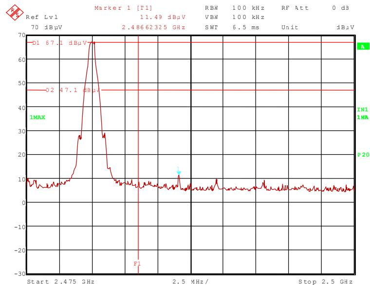
111592\_7.wmf: Radiated band-edge compliance, upper band edge, hopping on (operation mode 4):
