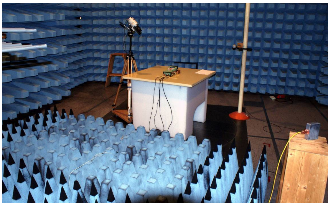
Photo 4: Measurement setup for radiated Immunity
