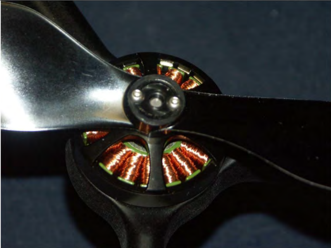
Picture 6: view into the propeller motor
