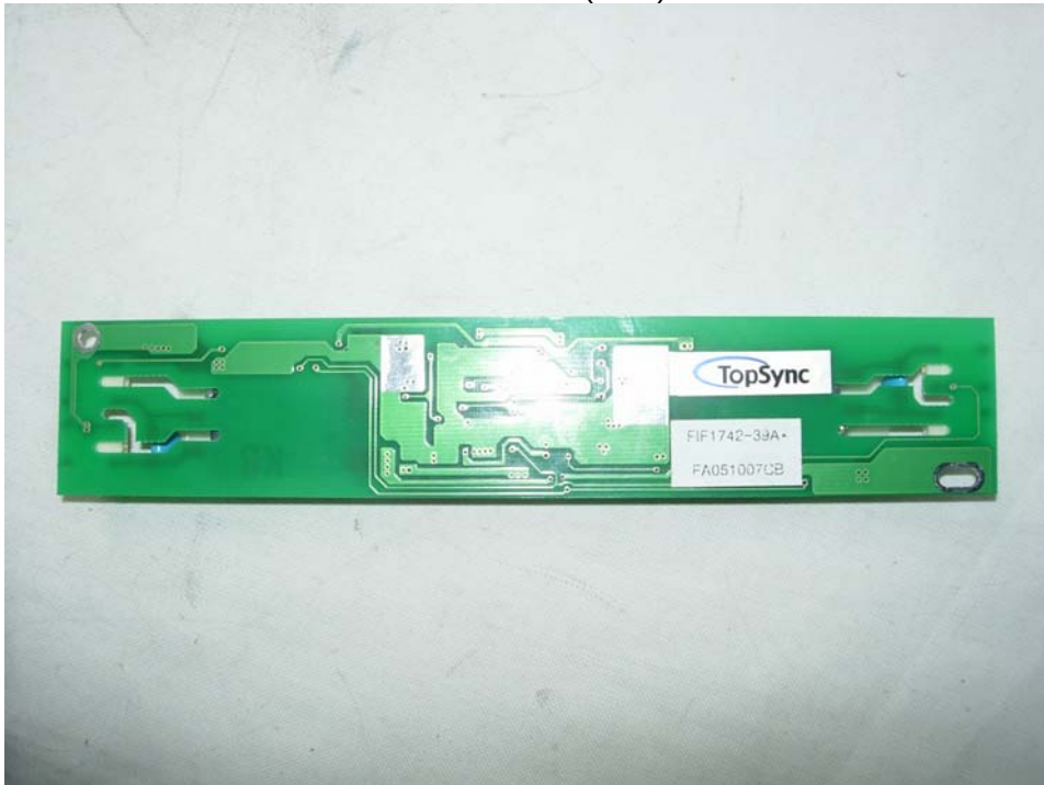
Inverter board (Rear)
