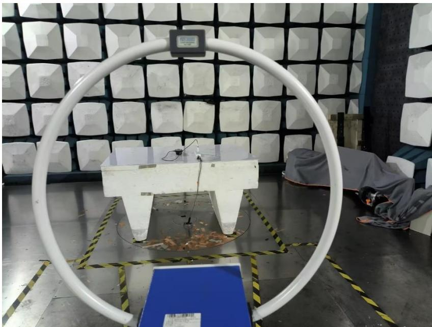
**Radiated Emissions (30MHz-1GHz)**
