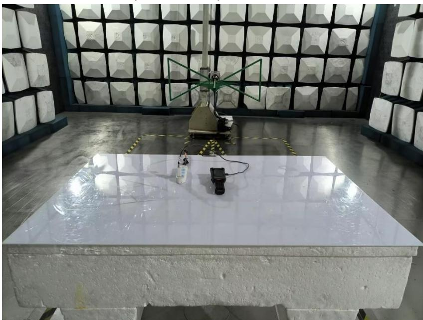
**Radiated Spurious Emissions Below 1GHz**
