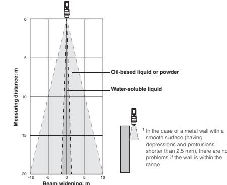
Detection may be unstable at close distances. Install the sensor or sensor head at the following recommended distances from the expected upper limit of the liquid level.
