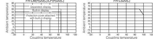
On the FR-LM20/LP20, selecting [Turns off when no op.] for "Screen brightness" can alleviate the ambient temperature regulation by 10°C.
