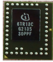
Wireless IC side (Black center IC is wireless IC)
