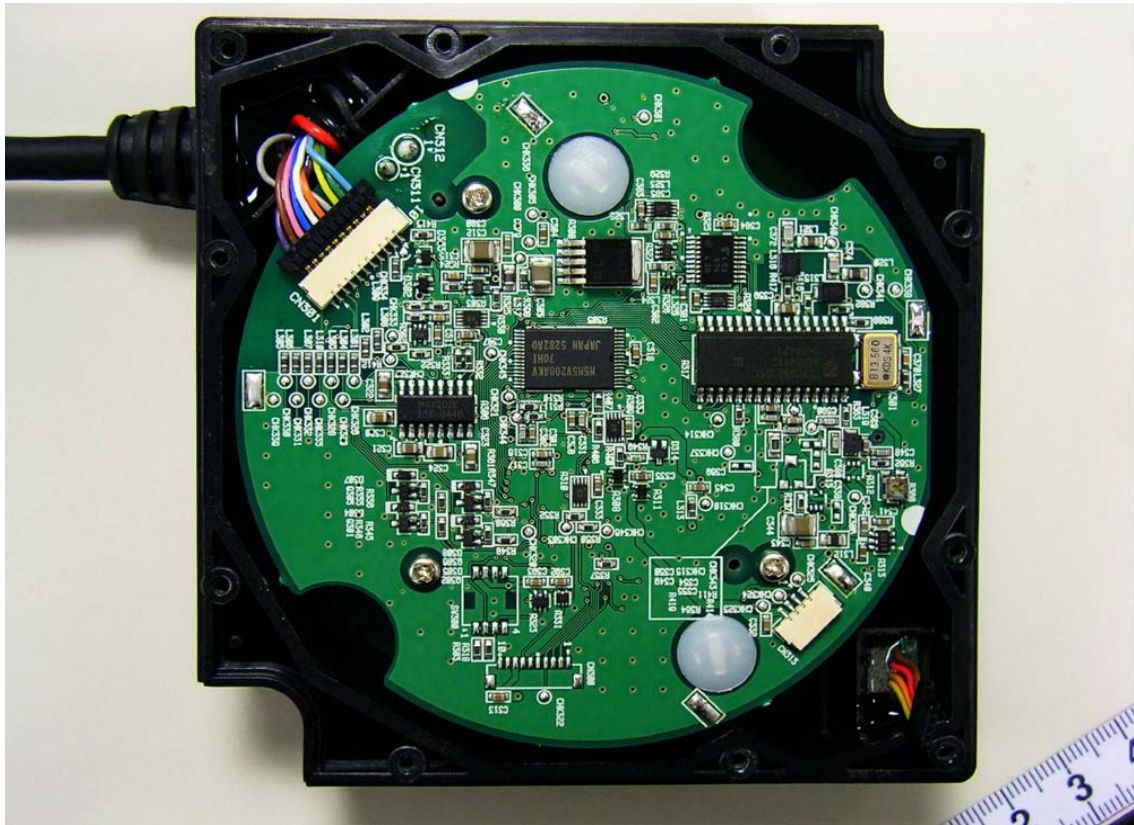
Internal View of RFID without Shield (Main Board)
