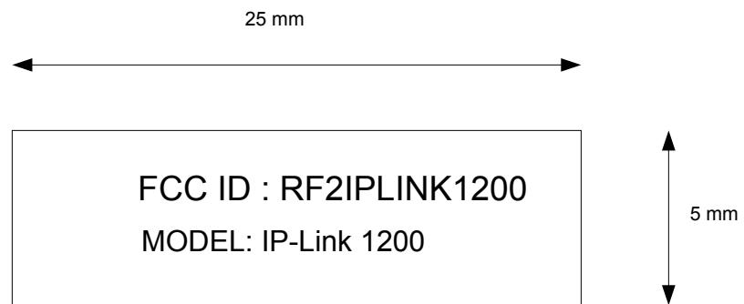
The above Label is located on top of the shield as shown below:
