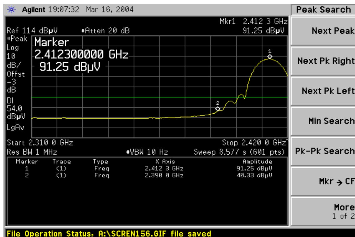
**Band Edges (802.11b / CH High)****Detector mode: Peak****Polarity: Vertical**
