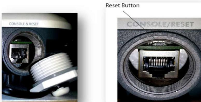
Reset button is above the console port RJ45 connector.
