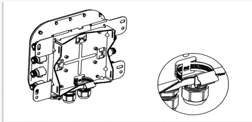
4. Lock and tighten the pole strap to secure the pole mount bracket to the pole.
