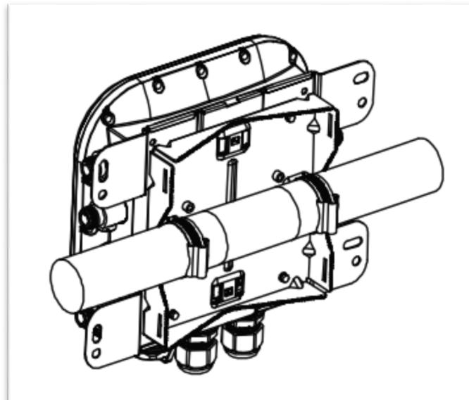
**Note:** The installation is correct if the node does not easily move from up and down.
