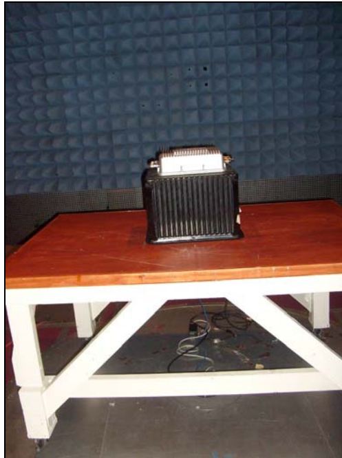
Photograph 2. Radiated Emission Spurious Test Setup
