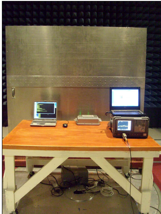
Photograph 5. Conducted Emissions, 15.207, Test Setup
