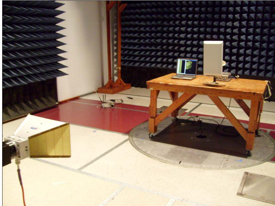
Photograph 9. Test Equipment and Setup for Various Radiated Measurements – 16 dBi Sector
