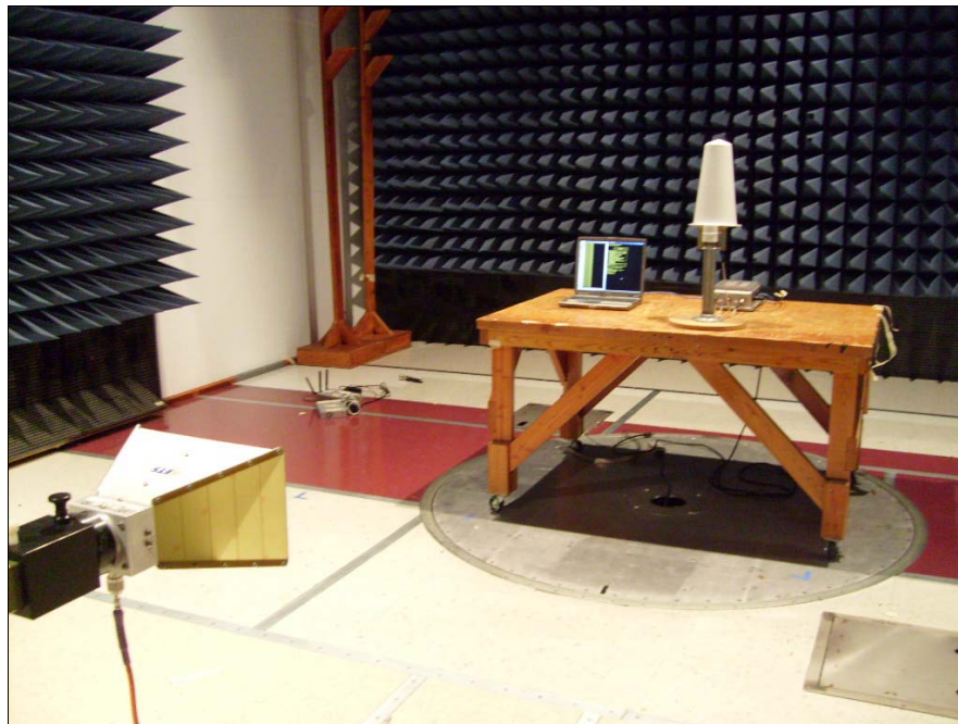
Photograph 7. Test Equipment and Setup for Various Radiated Measurements – 9 dBi Omni
