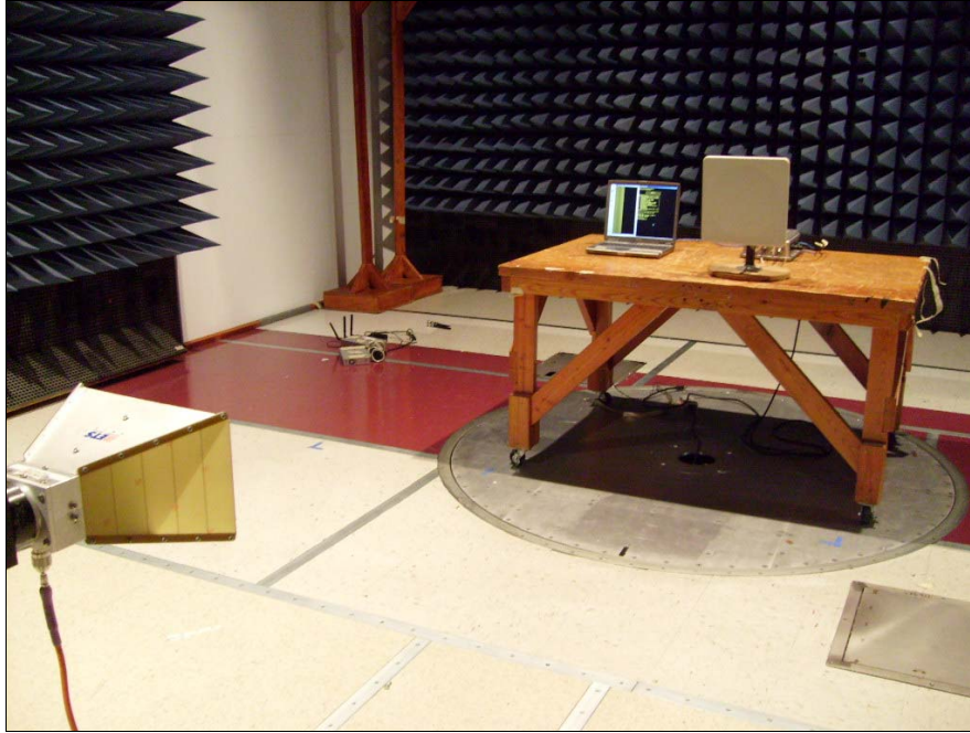
Photograph 10. Test Equipment and Setup for Various Radiated Measurements – 19 dBi Panel
