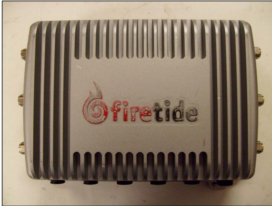
Photograph 1. Firetide, Inc., 7200 Outdoor Unit
