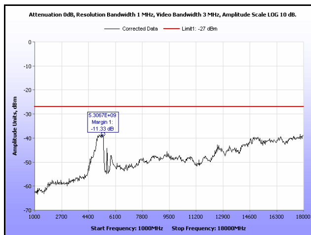
Plot 61. Radiated Spurious Emissions, 802.11n 20 MHz, 5580 MHz, 1 GHz – 18 GHz, 16 dBi Antenna
