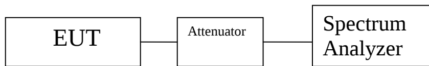
Figure 2. Block Diagram, Occupied Bandwidth Test Setup
