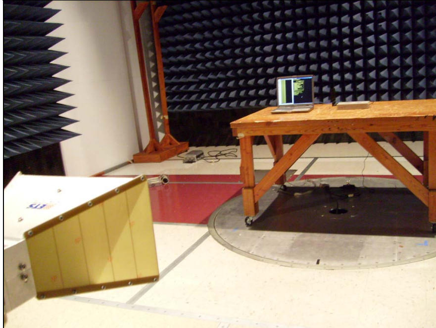
Photograph 7. Test Equipment and Setup for Various Radiated Measurements – Combined Omni Antennas
