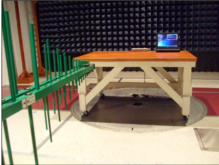
Photograph 4. Radiated Emission, Test Setup, 30 MHz – 1 GHz
