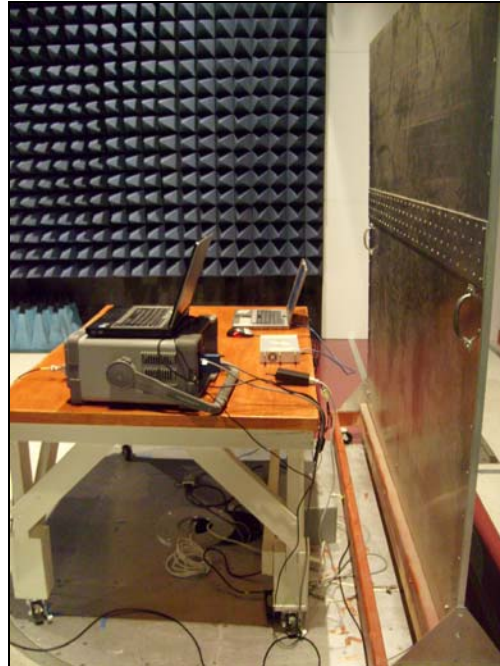
Photograph 2. Conducted Emissions, Test Setup. Side View
