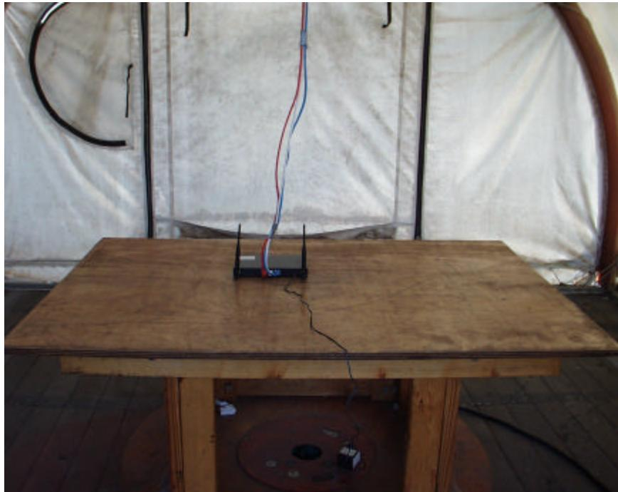
**DIGITAL DEVICE RADIATED EMISSIONS SETUP**
