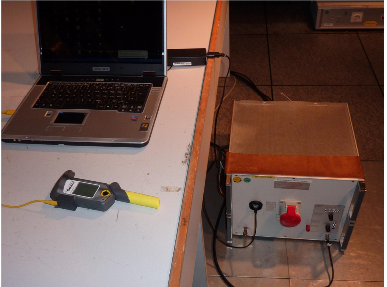
123379emi3.jpg: Test setup conducted emission
