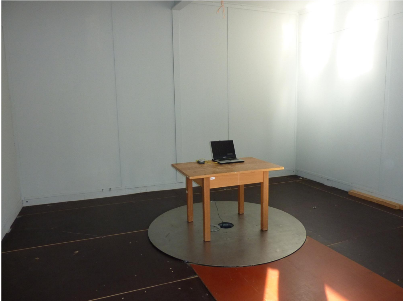
123379emi2.jpg: Test setup open-area-test-site OATS
