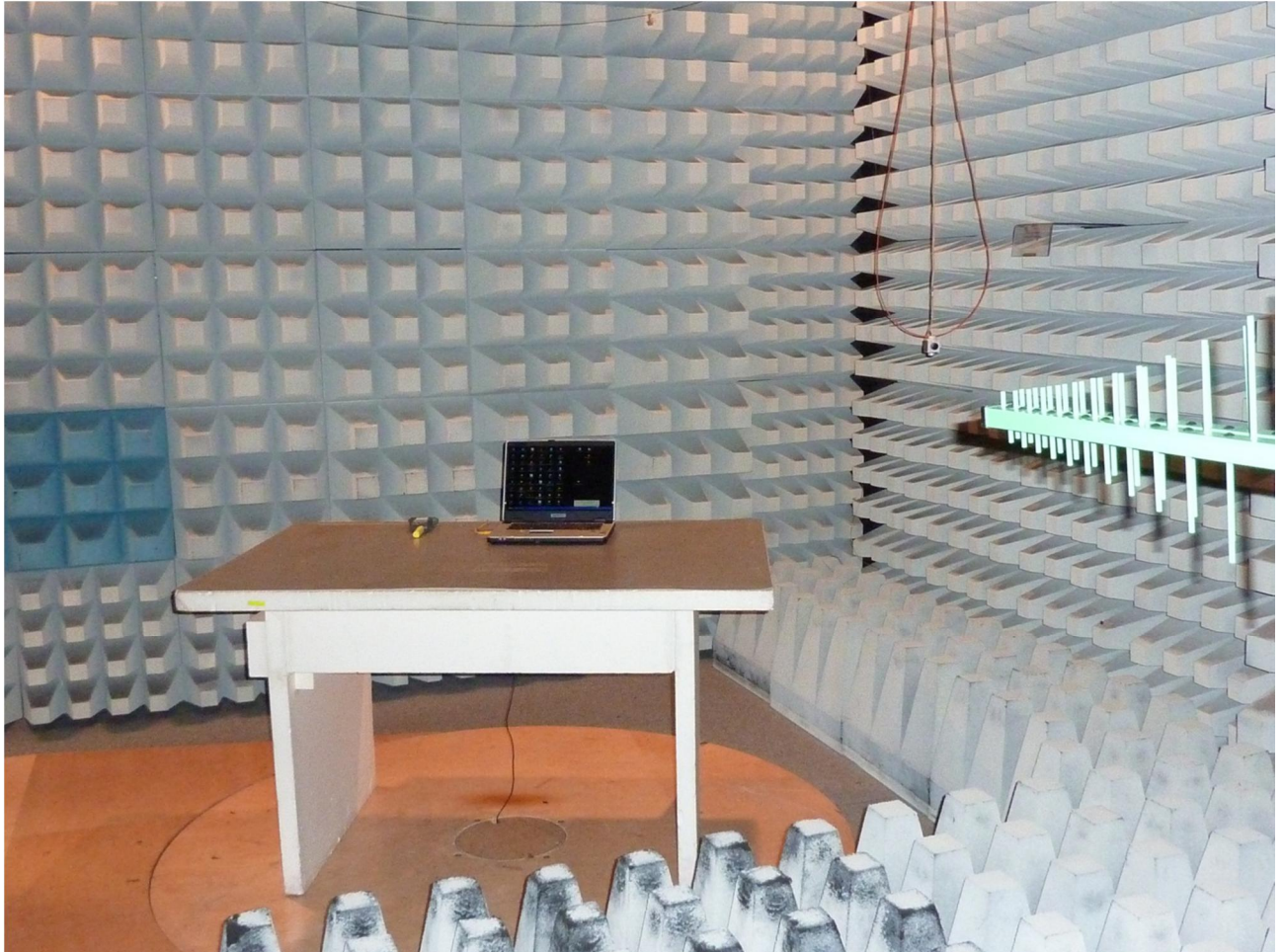
123379emi1.jpg: Test setup anechoic chamber
