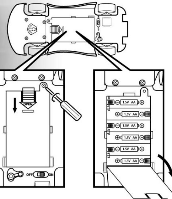
3) To open the car battery lid, use screwdriver to turn the screw in counter-clockwise.
