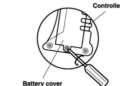
1) To remove the controller battery lid, use screwdriver to turn the screw in counter-clockwise.
