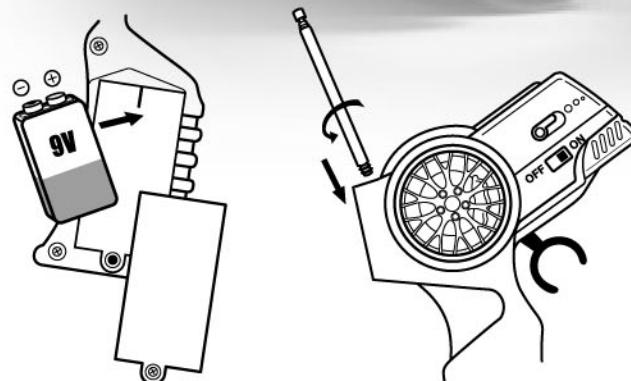
2) Install 1x9V size alkaline battery with polarity as shown inside battery compartment. Before operating the controller, make sure the antenna is fully extended.
