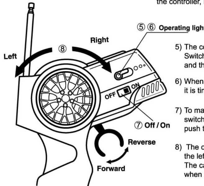
5) The controller is full function. Switch on the controller from off to on and the indicating light will come on.
