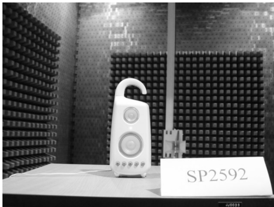
Photograph 3: Set-up for Radiation Measurement Above 1GHz
