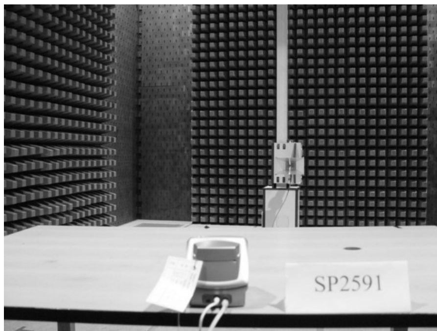
Photograph 3: Set-up for Radiation Measurement Above 1GHz
