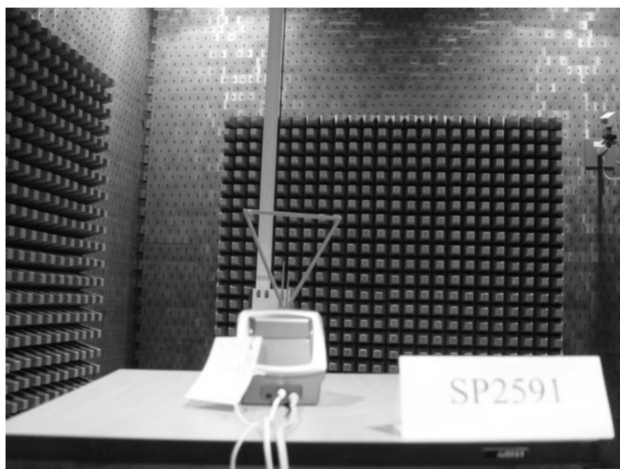
Photograph 2: Set-up for Radiation Measurement Below 1GHz
