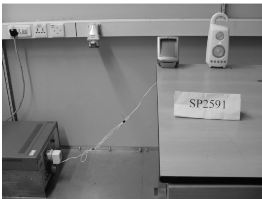
Photograph 2: Set-up for Radiation Measurement Below 1GHz
