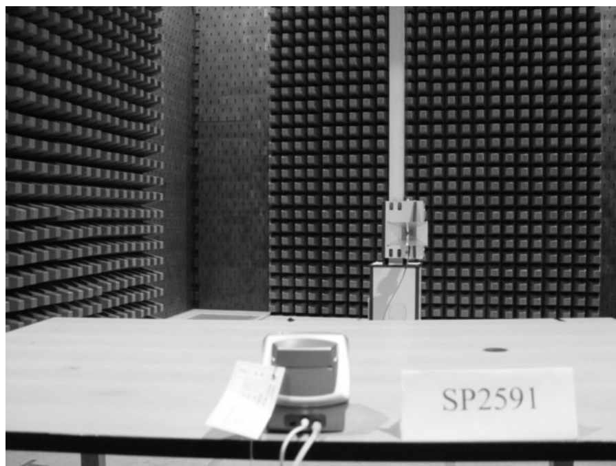
Photograph 3: Set-up for Radiation Measurement Above 1GHz
