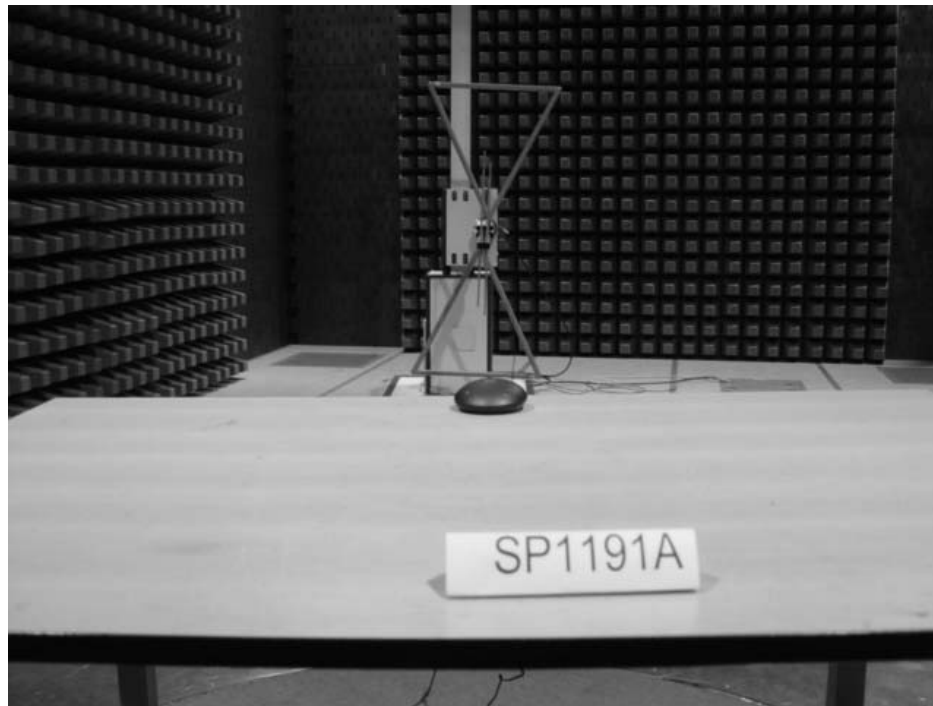
Photograph 2: Set-up for Radiation Measurement Below 1GHz
