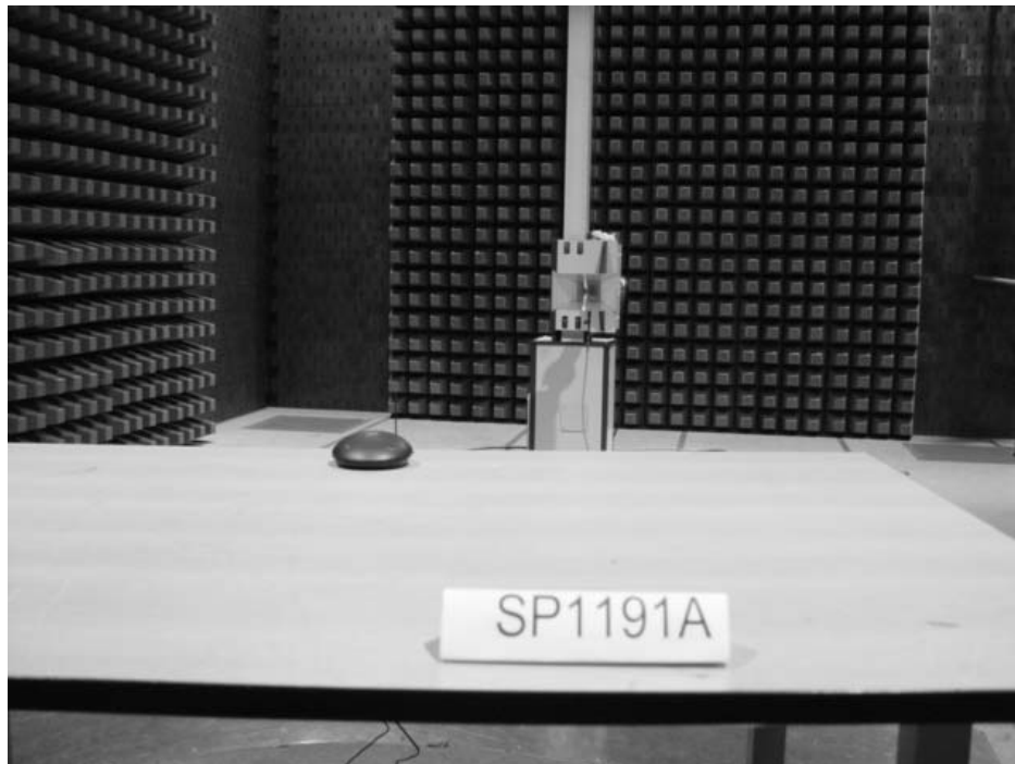
Photograph 3: Set-up for Radiation Measurement Above 1GHz
