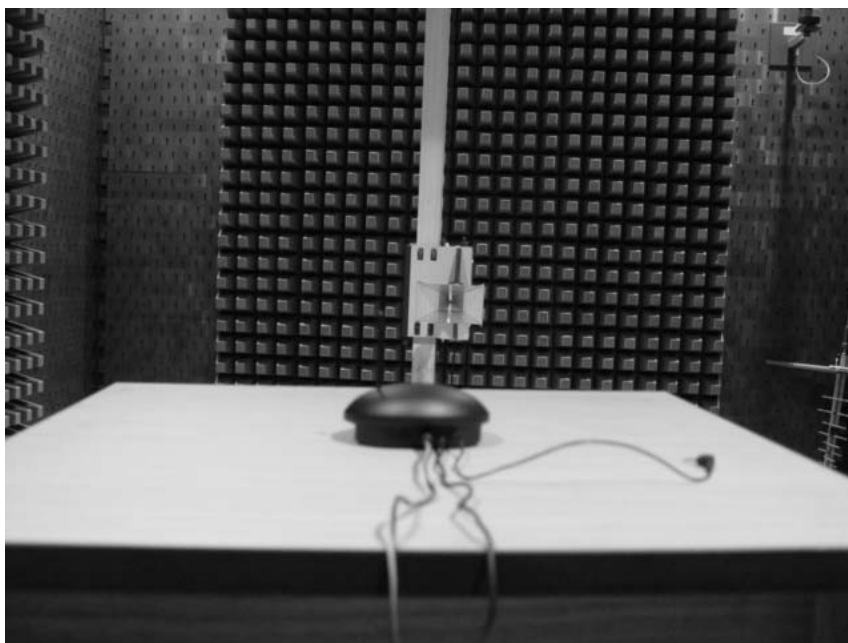
Photograph 3: Set-up for Radiation Measurement Above 1GHz
