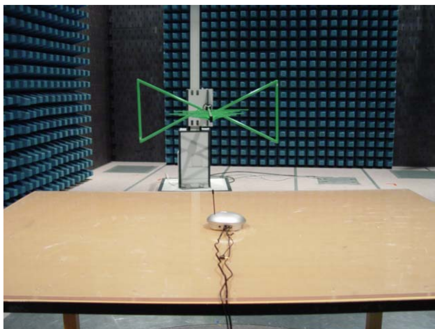
Photograph 2: Set-up for Radiation Measurement Below 1GHz
