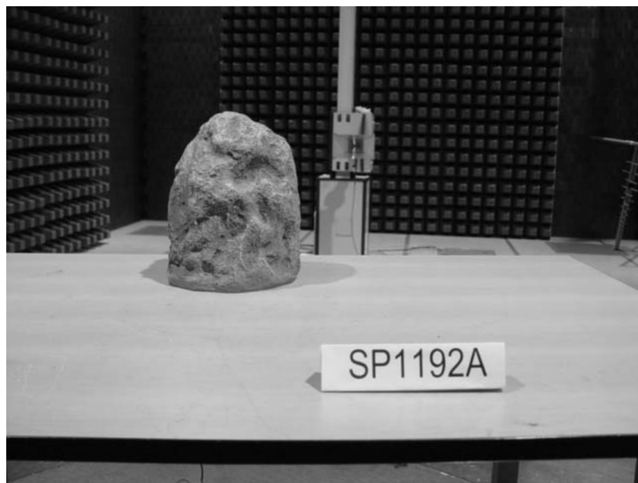
Photograph 3: Set-up for Radiation Measurement Above 1GHz
