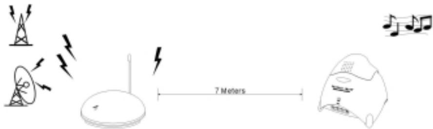
5. You should now be able to place the speakers freely from room to room without disruption. Should there is any disruption (signal cuts off or carries distortion), press the speaker's "AUTO TUNE" button to maximize the best reception.
