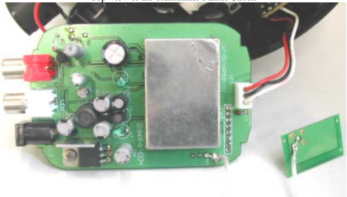
Top View of the Transmitter's Inner Circuit
