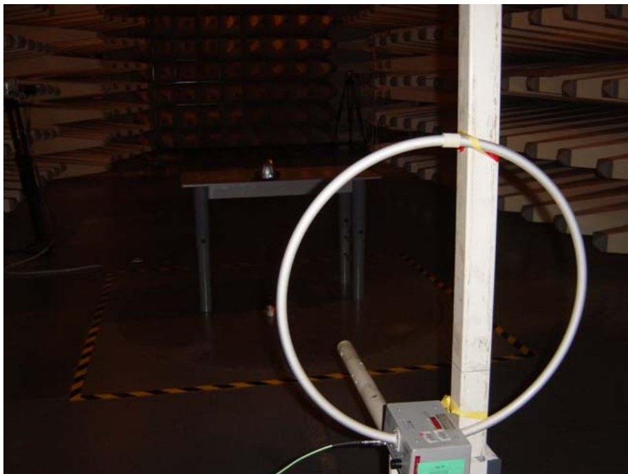
Radiated Emission Test
