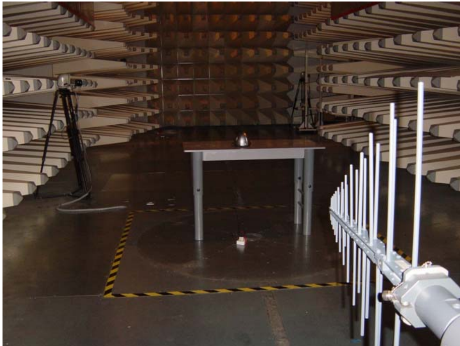
Radiated Emission Test
