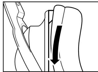
Turn the padding as illustrated. It will slide into the guide slot by itself. Keep turning it until it is correctly in place. Once it has taken on an oval shape, then it is correctly positioned.
