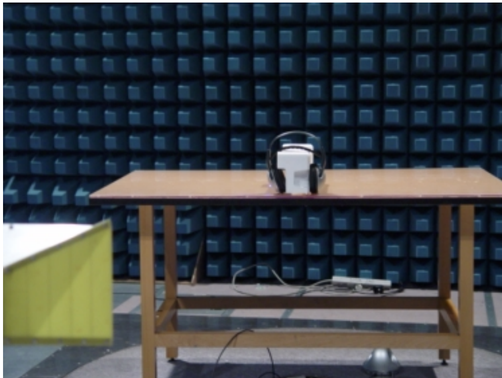
Photograph 2: Set-up for Radiation Measurement Above 1GHz
