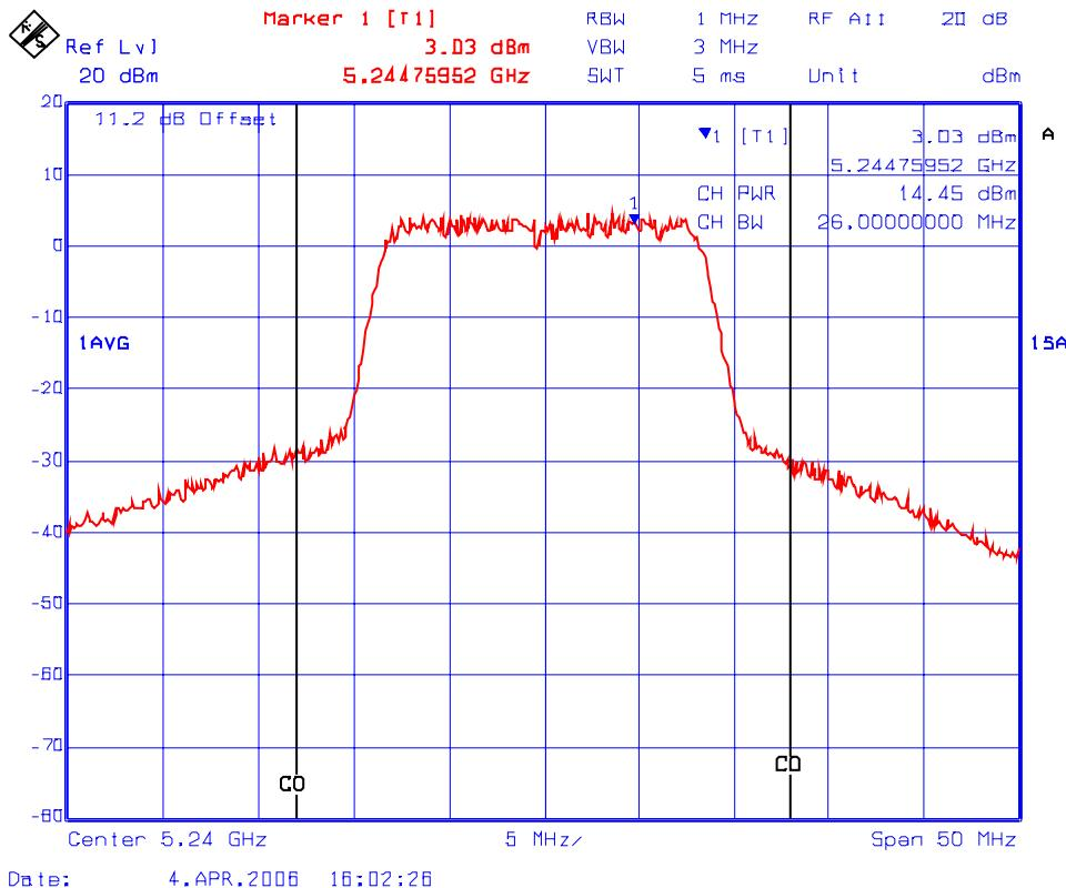
**Plot #4: Channel Conducted Power in 26 dB Bandwidth**
