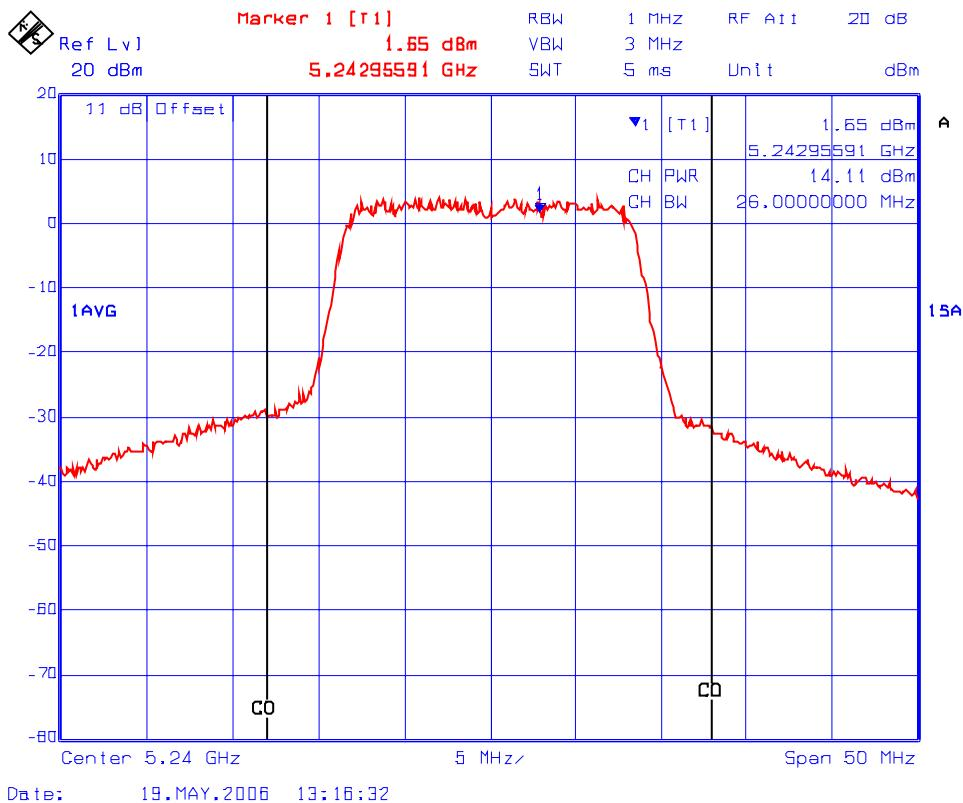
**Plot #13: Channel Conducted Power in 26 dB Bandwidth**
