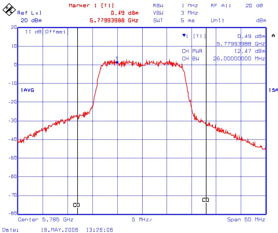
**Plot #18: Channel Conducted Power in 26 dB Bandwidth**
