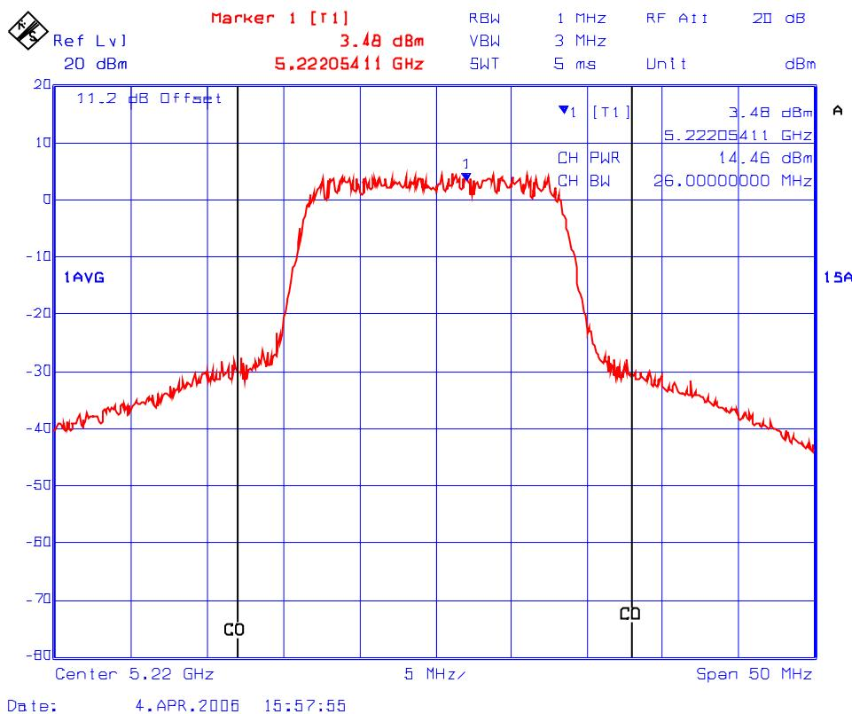
**Plot #3: Channel Conducted Power in 26 dB Bandwidth**
