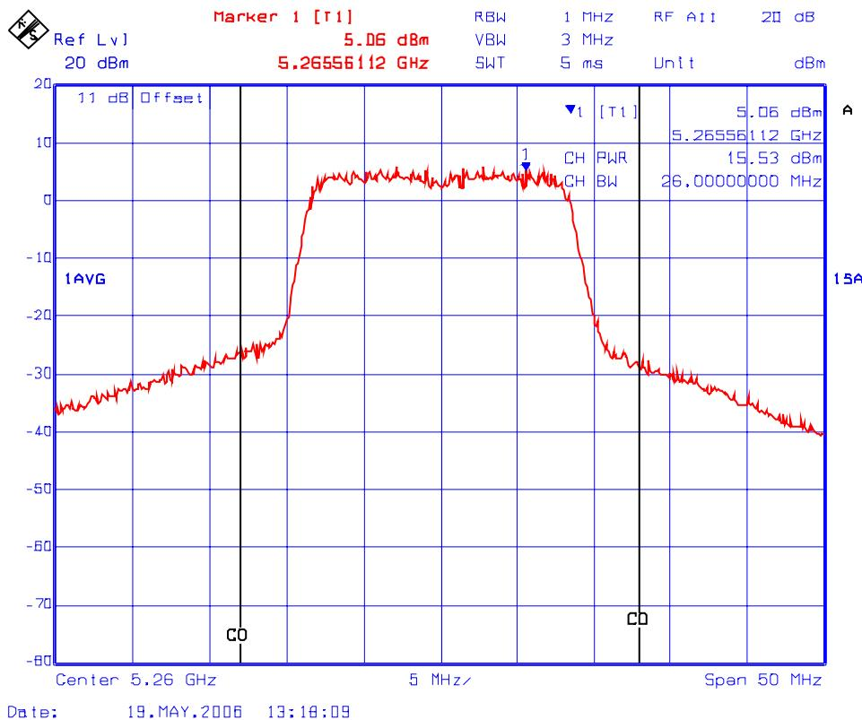
**Plot #14: Channel Conducted Power in 26 dB Bandwidth**
