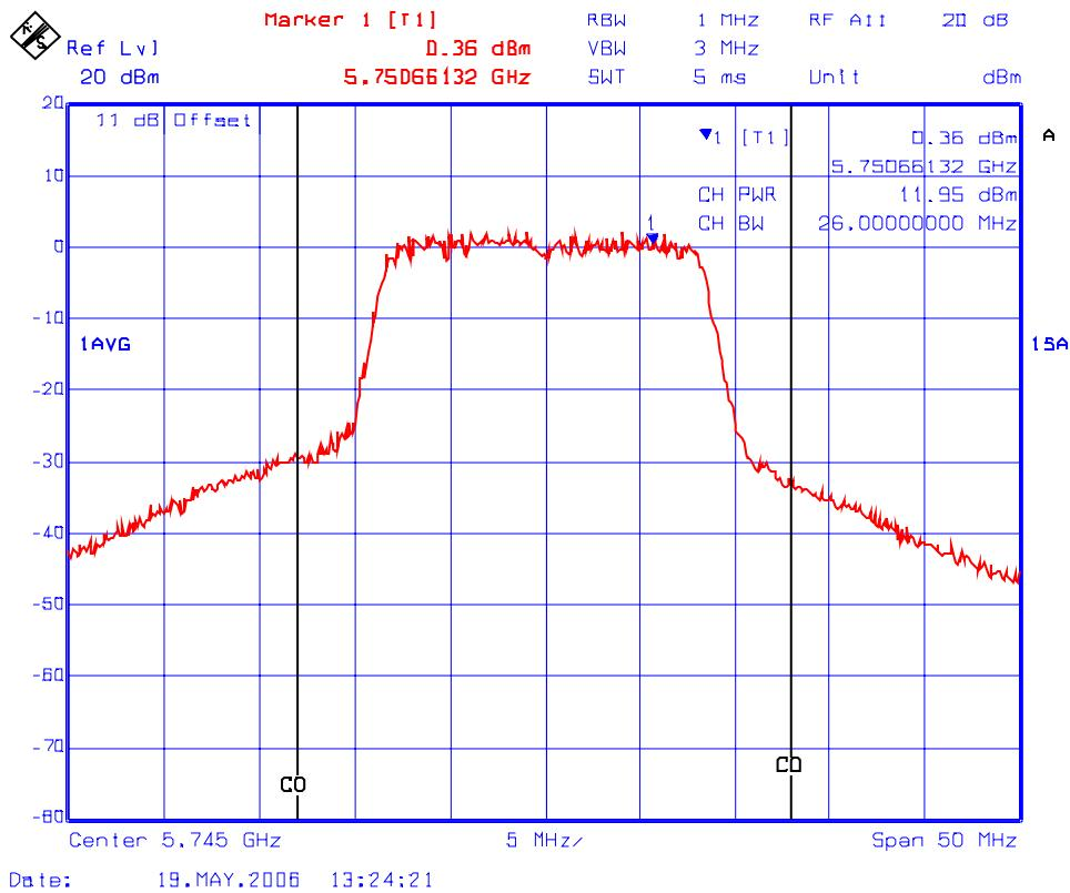
**Plot #17: Channel Conducted Power in 26 dB Bandwidth**
