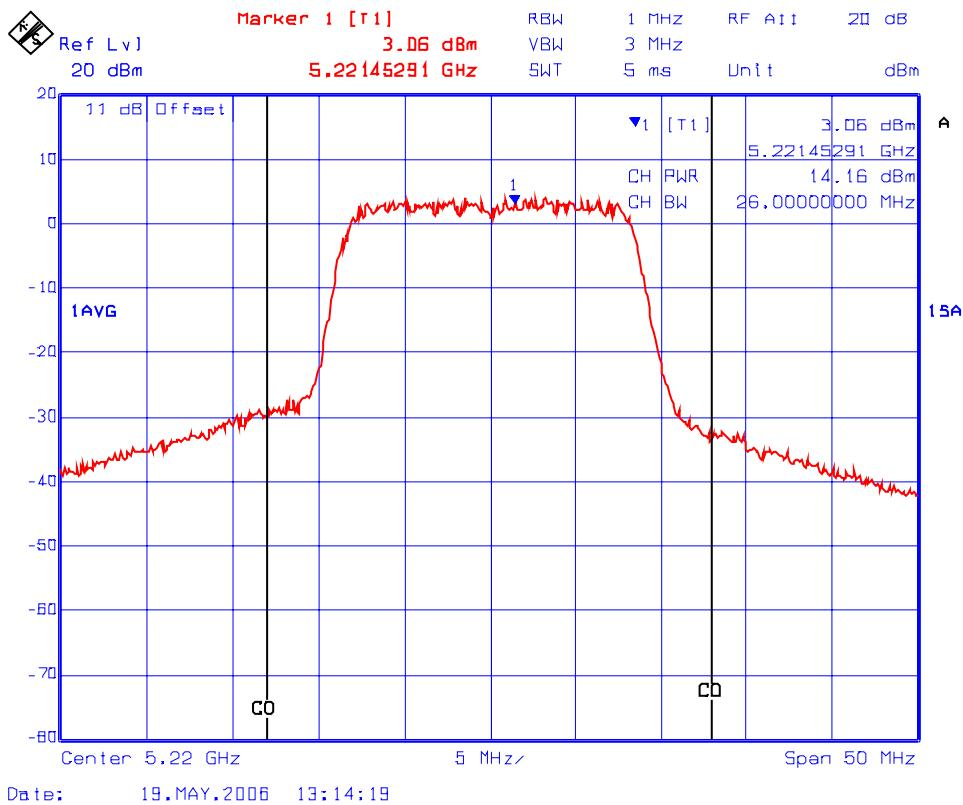
**Plot #12: Channel Conducted Power in 26 dB Bandwidth**
