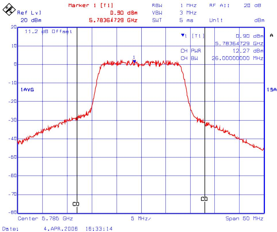
**Plot #9: Channel Conducted Power in 26 dB Bandwidth**
