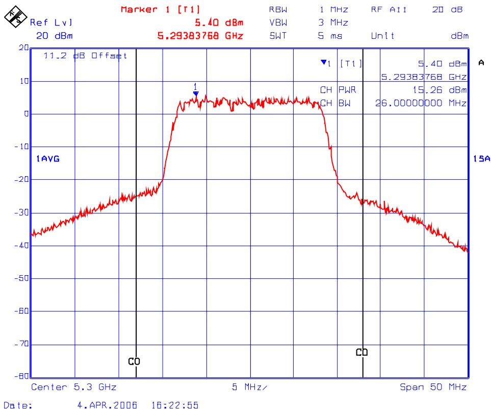
**Plot #6: Channel Conducted Power in 26 dB Bandwidth**
