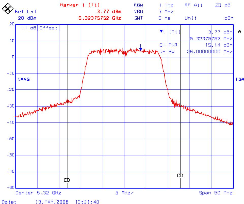
**Plot #16: Channel Conducted Power in 26 dB Bandwidth**
