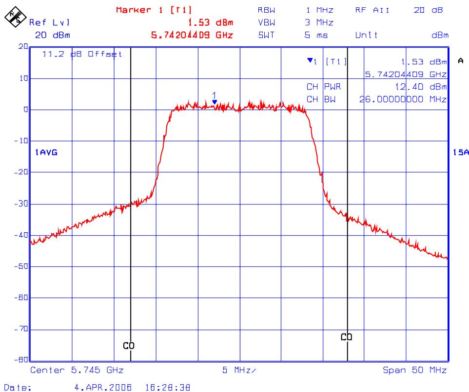
**Plot #8: Channel Conducted Power in 26 dB Bandwidth**
