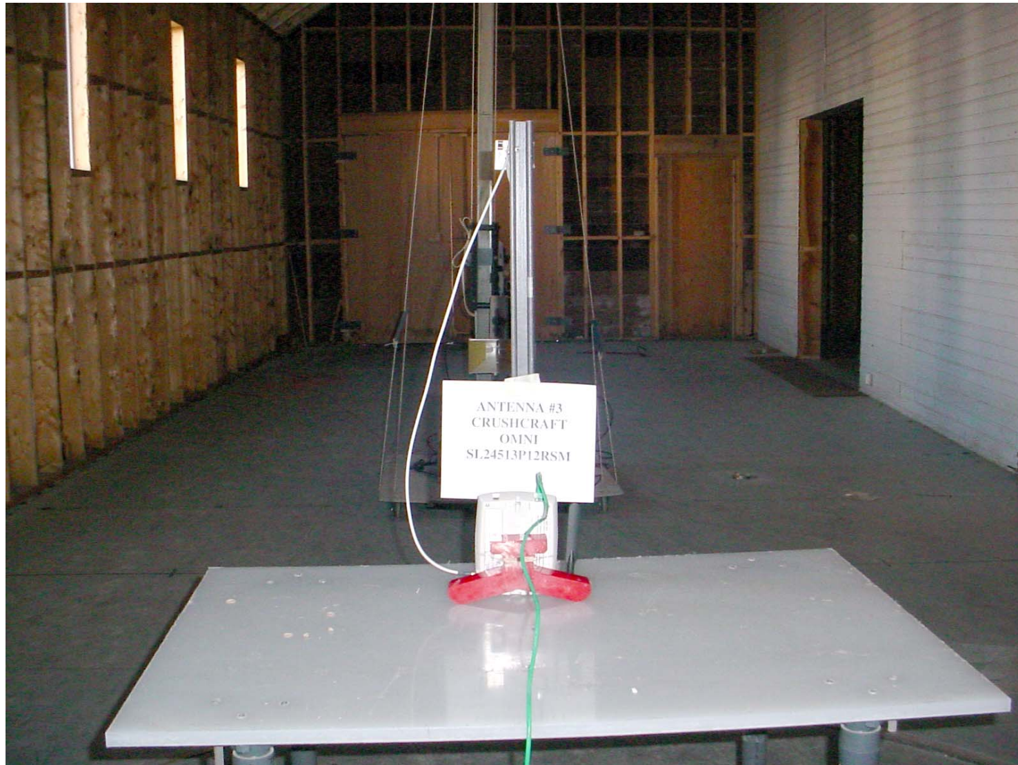
Photo #3b: HiPath Wireless Access Point with Cushcraft Omni External Antenna Model: SL24513P, 3 dBi gain
