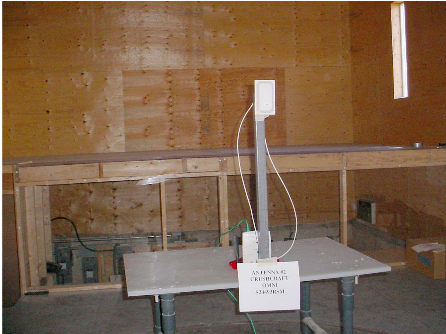
Photo #2a: HiPath Wireless Access Point with Cushcraft Omni, 2 Inputs External Antenna Model: S24493DS, 3 dBi gain
