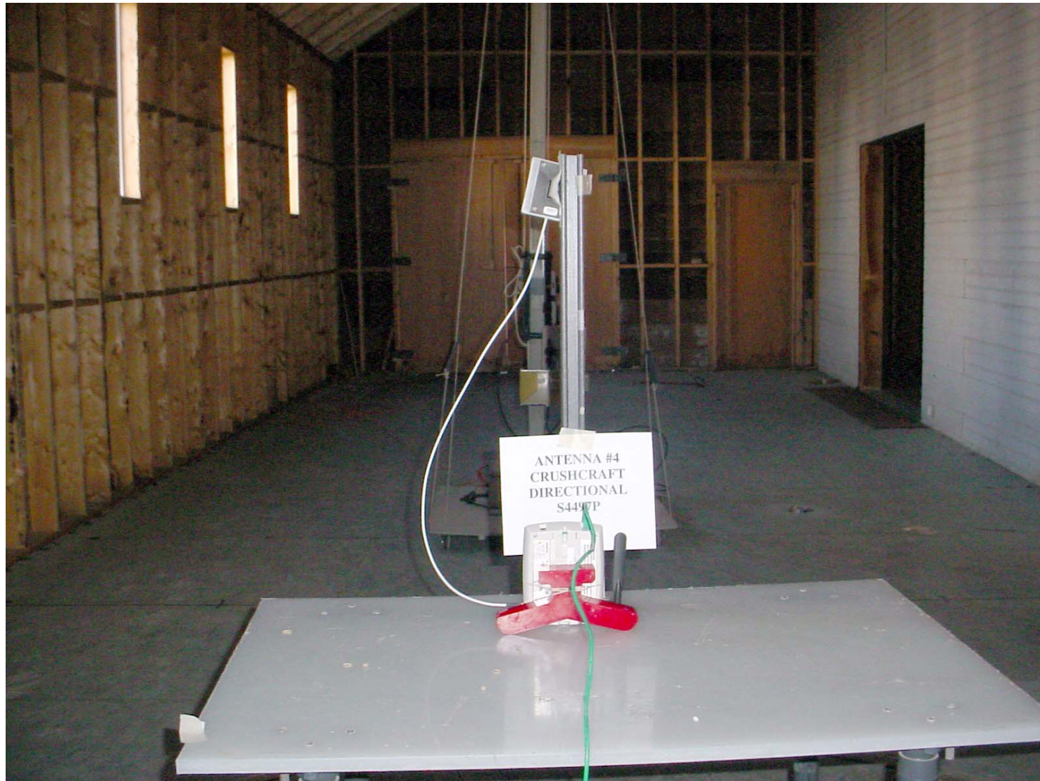
Photo #4b: HiPath Wireless Access Point with Cushcraft Directional External Antenna Model: S24497P, 7 dBi gain
