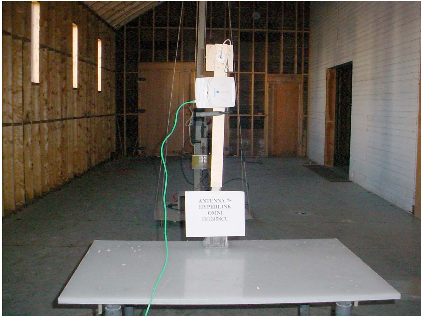
Photo #5b: HiPath Wireless Access Point with Hyperlink Technologies Omni External Antenna Model: HG2458CU, 3 dBi gain
