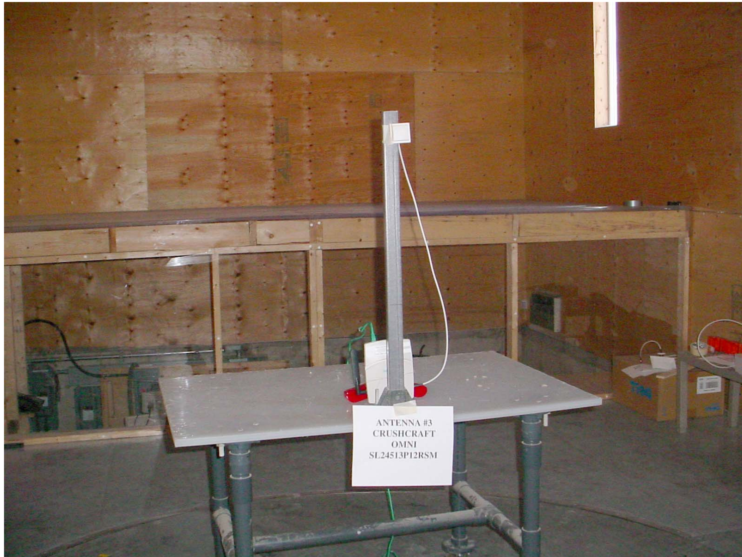
Photo #3a: HiPath Wireless Access Point with Cushcraft Omni External Antenna Model: SL24513P, 3 dBi gain
