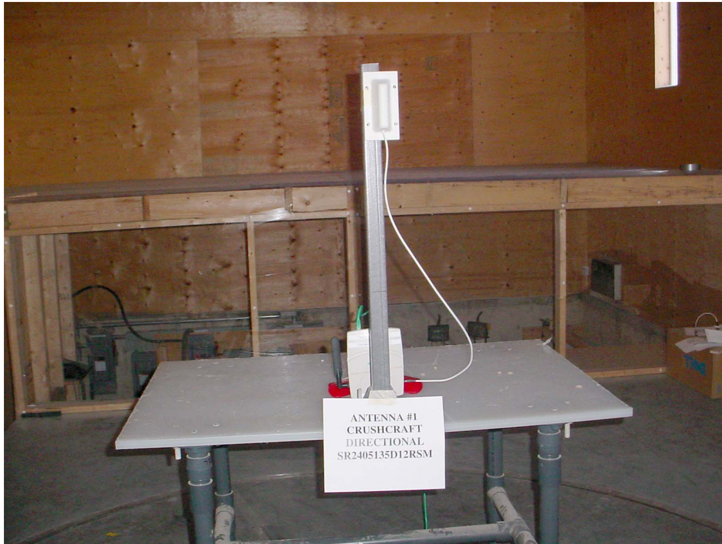
Photo #1: HiPath Wireless Access Point with Cushcraft Directional External Antenna Model SR2405135D, 5 dBi gain
