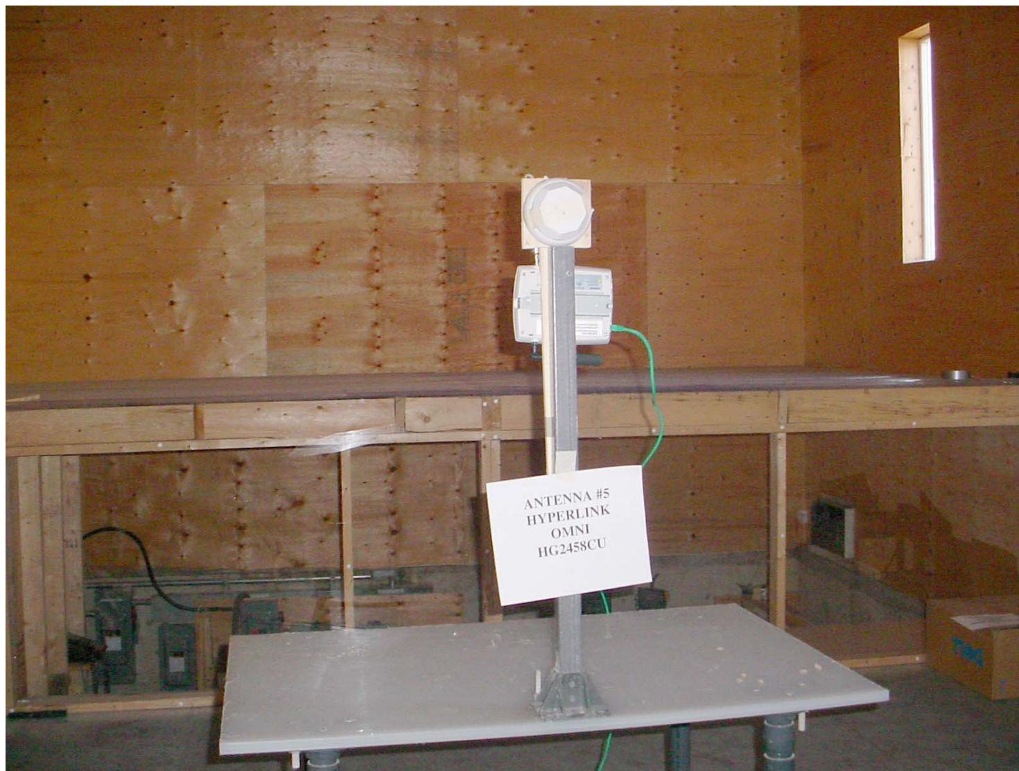
Photo #5a: HiPath Wireless Access Point with Hyperlink Technologies Omni External Antenna Model: HG2458CU, 3 dBi gain
