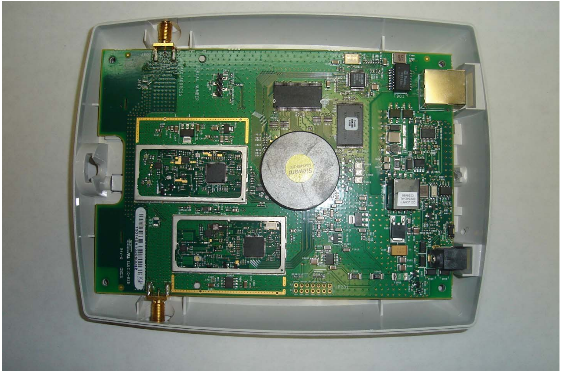
Model AP2620/AP2640 with external antennas wrt. reversed SMA connector
