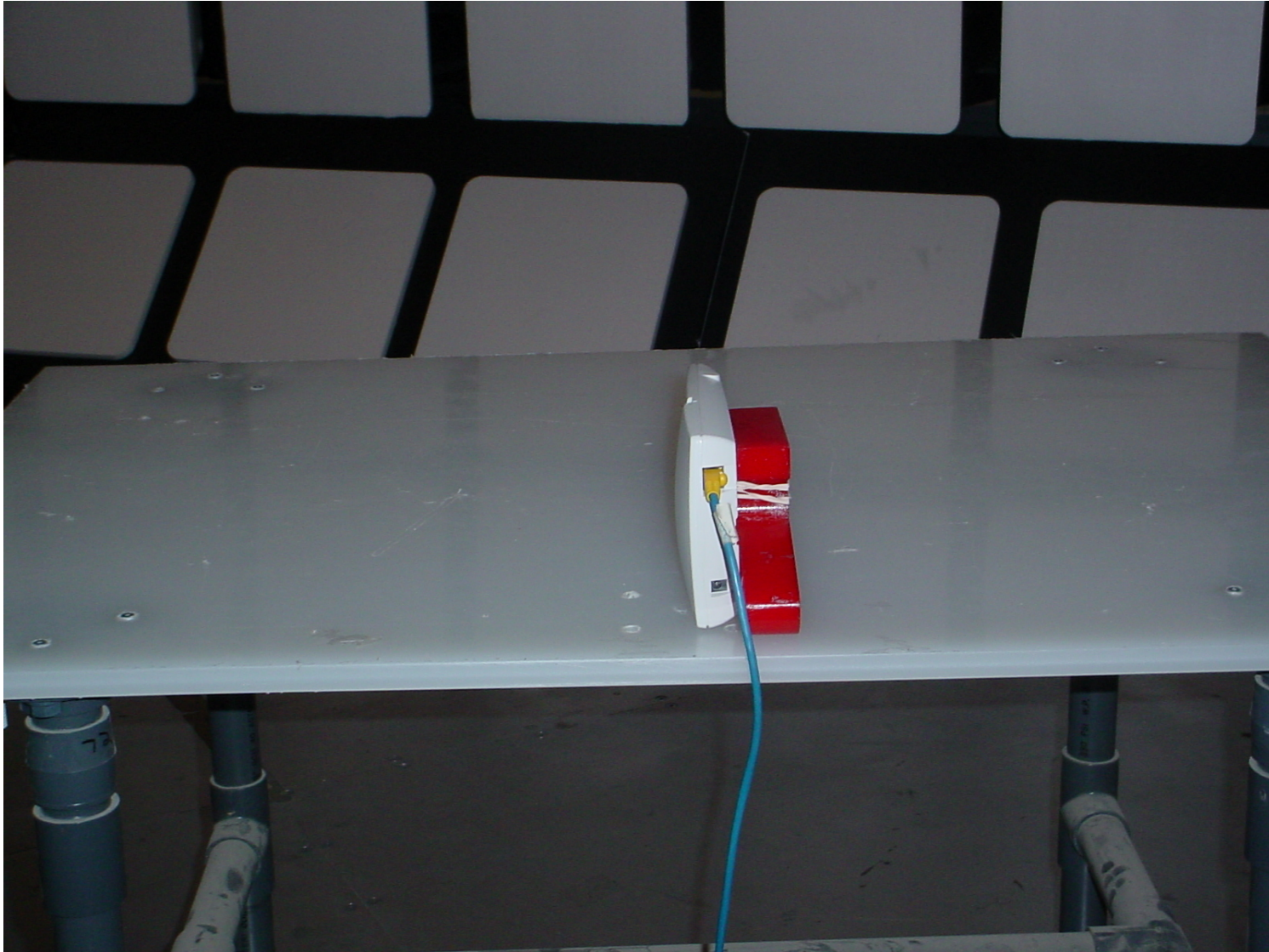
Photo #2: HiPath Wireless Access Point with internal antennas – Test Orthogonal Position #2
